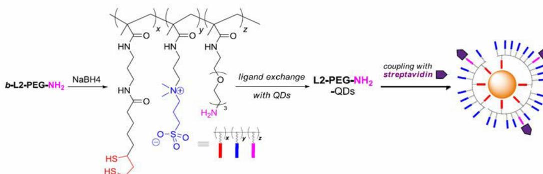
**Figure 5.1 : Schematic representation of ligand exchange and conjugation of QDots to streptavidin [106]**
