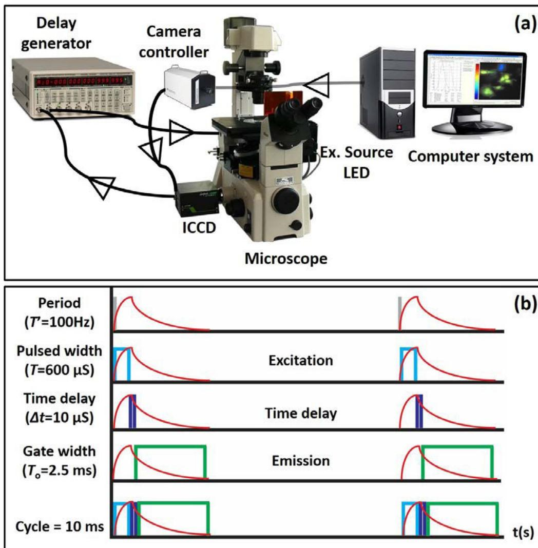
**Figure 4.3 : TG-FRET Microscopy setup.** (a) Experimental setup of TG-FRET relying on an epifluorescence microscope with an excitation LED light source emitting in UV range, an intensified CCD array detector (ICCD) and a delay generator to synchronize the acquisition. (b) Pulse sequence of TG-FRET including the duration of each pulse.
