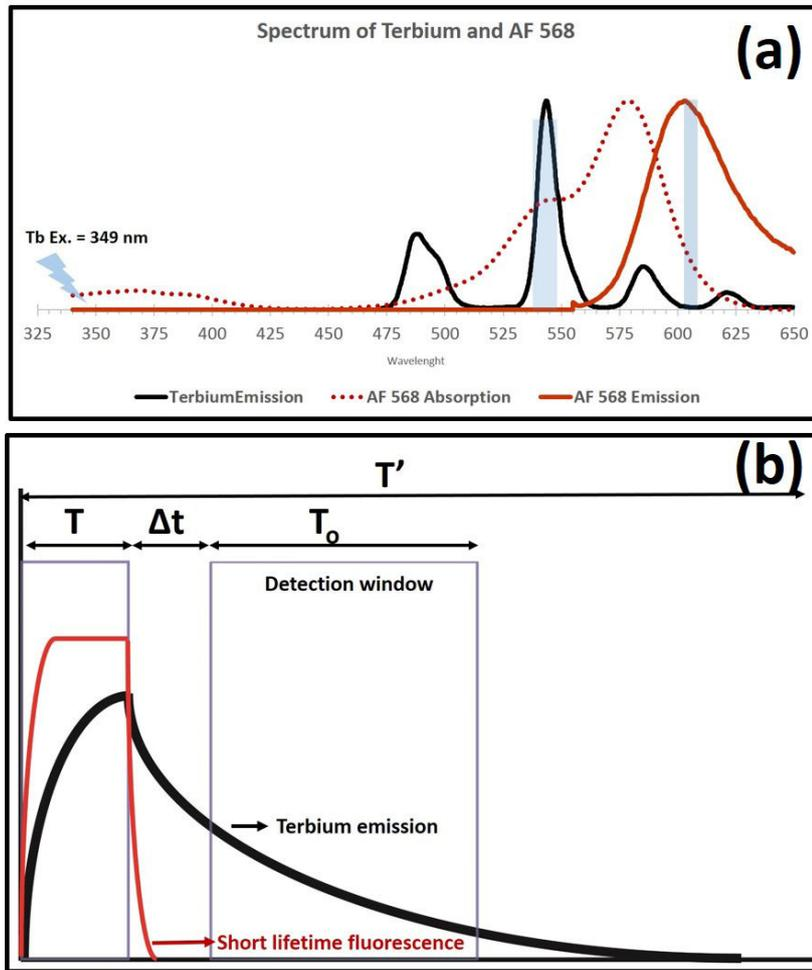
**Figure 4.2 : Schematic representation of TG-FRET detection.** (a) Terbium complex donor fluorescence spectrum (black) after excitation at 365 nm wavelength. Absorption (irregular red line) and emission (regular red line) spectra of AF568 acceptor. Bandpass filter detection range is displayed in light blue. (b) Principle of time-gated FRET.
