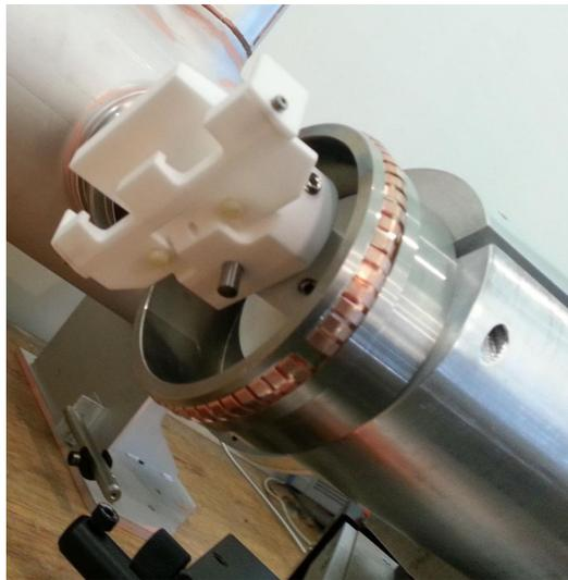
Figure 6.14: Alternative holder design, based on the initial metallic holder, except that all the parts seen by the beam were replaced by ceramic.
