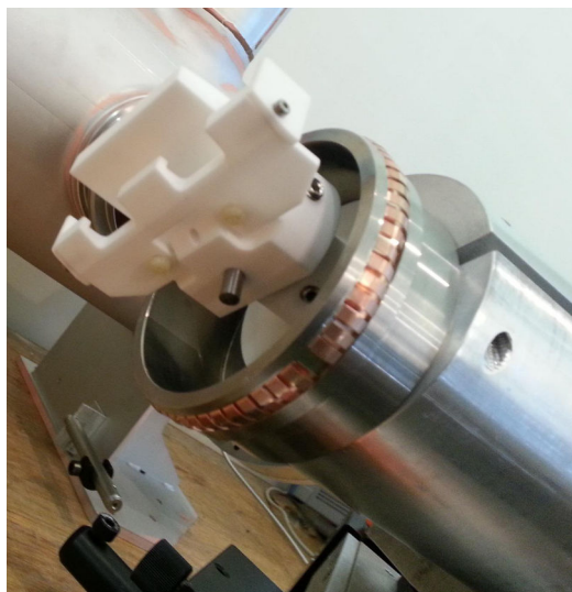
Figure 6.14: Alternative holder design, based on the initial metallic holder, except that all the parts seen by the beam were replaced by ceramic.
