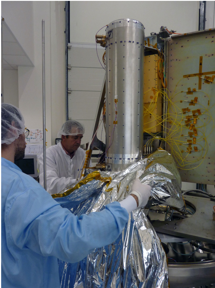
Figure 4.29: Vertically positioned PHARAO cesium tube before being wrapped by a thermal blanket and out into a vacuum chamber.
