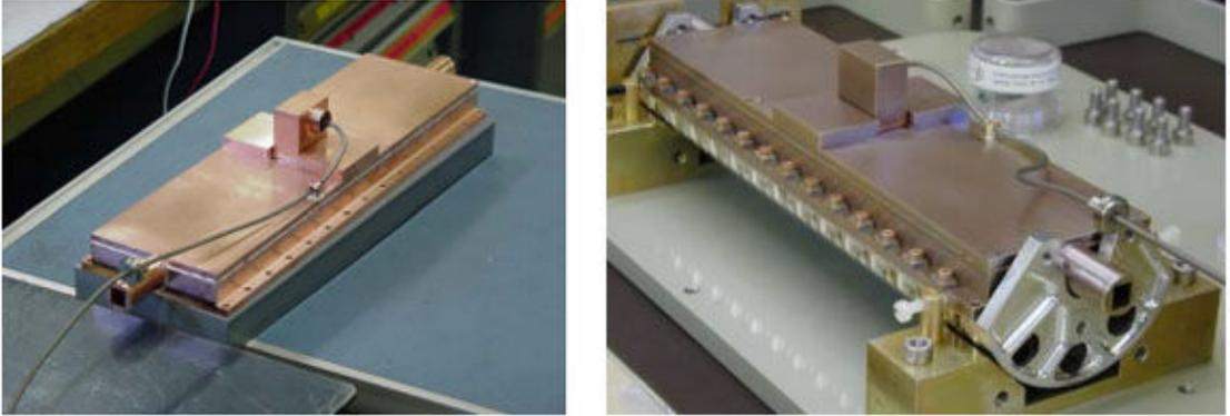
**Figure 4.21:** PHARAO flight model interrogation cavity and its supporting structure (on the right).
