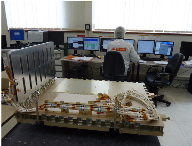
Figure 4.31: Ground segment used to send TC, receive TM and examine data with the software package MARIA.
