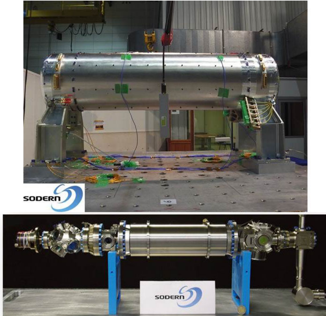
Figure 4.5: Flight model cesium tube with shields during vibrational testing (up) and the vacuum chamber (bottom).
