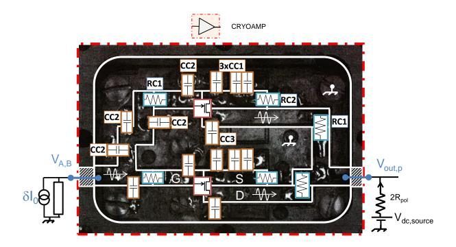
FIGURE 2.2 – Schematic representation of the 2-HEMT cryo-ampliphifier. Simplified version of the input and output circuits are represented. Stricly duplicated electronics has not been labeled on the bottom line. Real-size  $1.8\,\mathrm{cm} \times 2.8\,\mathrm{cm}$ .
