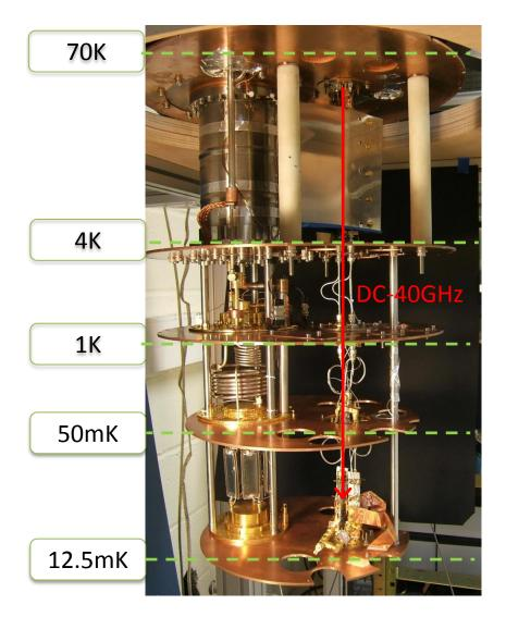
FIGURE A.2 – Cryogenic System. Helium-Free  $400\mu W$  with base temperature 12.5mK from Cryoconcept<sup>TM</sup>. The Photo adapted from [37]. Distances between the stage are -from 70K to 12.5mK- 25cm-10cm-15cm.
