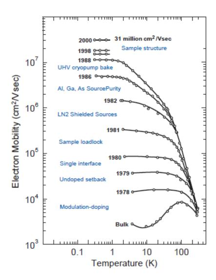
FIGURE B.2 – History of improvements in the mobility of electrons in GaAs, annotated with the technical innovation responsible for the improvement. From Pfeiffer et al.[116].
