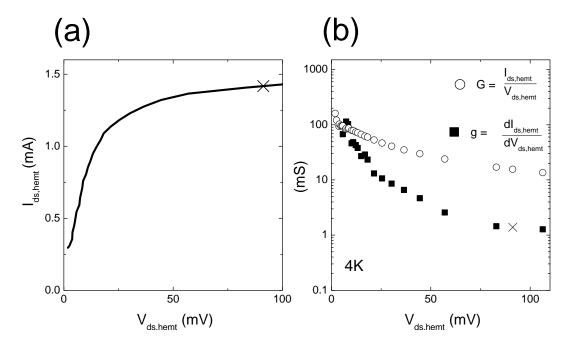
FIGURE 2.3 – On both (a) and (b), the cross marks the selected working point. (a) Drain current  $I_{\rm ds,hemt}$  as a function of drain-source voltage  $V_{\rm ds,hemt}$  for each self-polarized ATF-34143 in the 2-HEMT device. Measurement is performed in an He<sup>4</sup> bath. (b) Black dots represent  $G(V_{\rm ds,hemt})$  the non-linear conductance of the channel at 4K. Black squares represent the constrained differential conductance  $g=dI_{\rm ds,hemt}/dV_{\rm ds,hemt}$ .
