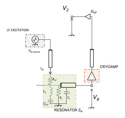
FIGURE C.1 – Joule Heating generation in measurement resistors. The current  $I_{dc}$  used to generate a bias on the quantum conductor also circulates in the resistors  $R_{LF}$  and  $R_{L}$ . When the QPC is pinched, we can observe how it affects the sample measurement.
