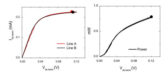
FIGURE F.3 – (a) Drain current  $I_{ds}$  as a function of drain-source voltage  $V_{ds}$  for a each ATF-34143 in a 10-HEMTs amplifier. Two prototypes were tested, leading to the red and black curves, both in an He<sup>4</sup> bath. Values are derived from the total  $I_{ds}(V_{dc})$  measurement, and then interpreted as an individual I-V curve. A dot marks on each curve the polarisation point used for the noise calibration. (b) Total power consumption.
