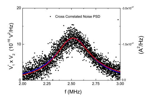
FIGURE 2.9 – Cross-correlated amplified noise spectral noise density filtered by the resonant circuit (black dots). The QPC with transmission 0.32 is biased with  $90\mu$ V. The equilibrium noise spectrum has been substracted. Each data point corresponds to an average over 60000 PSD spectra. Best fit with exact shape (red curves) and Lorentzian approximation (blue curve). The original computed spectrum has a negative sign which has been removed.
