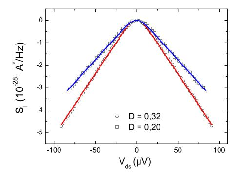
FIGURE 2.11 – Shot Noise DC with heating effect for low-transmission gain calibration. Two experimental transmissions are used D=0.2 (square dots) and D=0.32 (round dots). Each data point corresponds to an ON-OFF procedure and to thus twice 60000 PSD spectra. Fits with the same adjusted cross correlation gain and electronic base temperature are plotted (blue and red line). Heating effects are estimated using the model from Kumar et al. [78]
