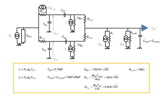
FIGURE 2.28 – Small signal model of amplification line with two parallel transistors in the MHz range.
