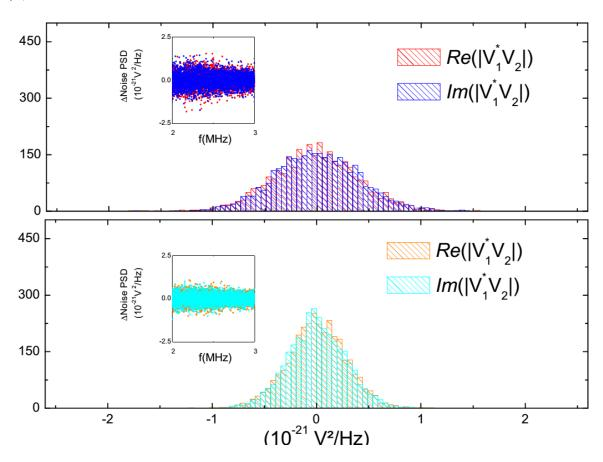
FIGURE 2.24 – Histograms of cross-correlation ON-OFF measurement with  $N_{av}$ =20000 (top part) and  $N_{av}$ =20000 (bottom part), and real (red-orange dots) and imaginary (blue-cyan dots). Data points are obtained from the difference  $\Delta NoisePSD$  of two successive measurements in identical conditions (Insets). All results are input-referred to eliminate gain discrepancies.
