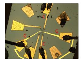
FIGURE B.6 – Optical image for Sample "B". Two bonding wires are used for each contact pad to decrease the parasitic inductance/resistance. Real-size  $1\,\mathrm{mm}\times1\,\mathrm{mm}$
