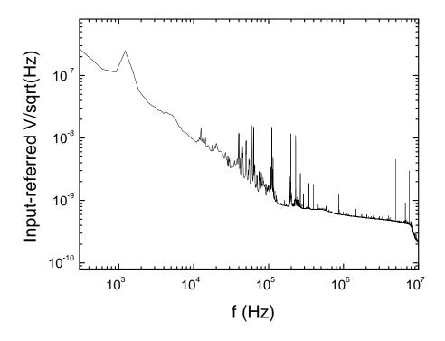
FIGURE C.9 – Input-referred spectral noise density from post- amplification. The amplifier model is NF SA421SA. A short circuit is placed at the input of the splitter board. The white noise observed in the range 1-10 MHz is in agreement with manufacturers specifications.
