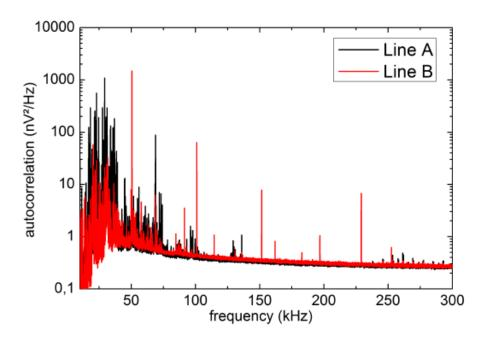
FIGURE 2.20 – Full Auto-correlations spectrum showing the amplified spectral noise density for acquisition line A (black) and B (red) with a full room-temperature amplification system (gain $\sim$ 80000) and DC $\sim$ 200 kHz in the Cryoconcept Helium-free cryostat. Almost all peaks in the DC $\sim$ 50 kHz band were observed to disappear when the cryocooler was turned off. From [37].
