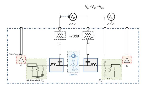
FIGURE 3.1 – RF Injection lines. The two lines are built from the same plan and can be both used. In practice, the detailed calibration reported here refers only to one of them, used for single pulse injection experiments.
