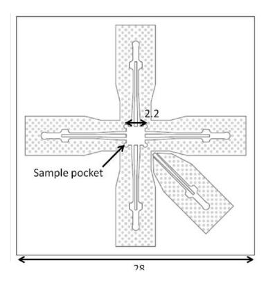
$\ensuremath{\mathsf{Figure}}$  D.1 – Sample holder. Dimensions are in mm.
