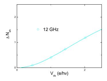
FIGURE 3.4 – In-situ calibration of AC amplitude at  $\nu = 12\,\mathrm{GHz}$ .
