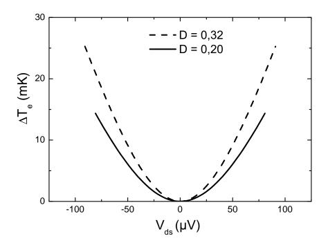
Figure 2.12 – Electron heating in noise calibration.
