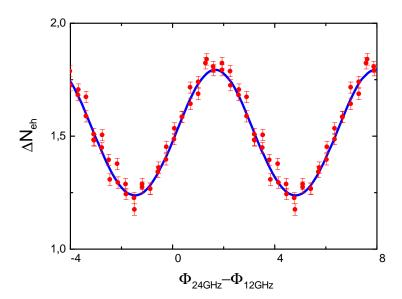
FIGURE 3.10 – Control of Relative Phase between second and fourth harmonic.  $\nu_0 = 6 \,\text{GHz}$ . Experimental parameters :  $q \sim 1.17$ ,  $\alpha_2 \sim 1.81$  and  $\alpha_4 \sim 0.68$ . This values gives large noise and large contrast. The best fit is based on a full photo-assisted calculation, with a single adjustable parameter : the relative phase induced along the line.
