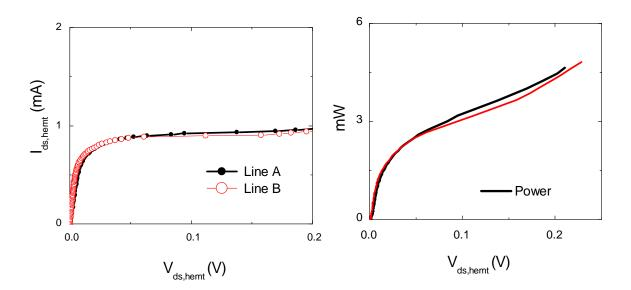
FIGURE F.6 – (a) Drain current  $I_{ds}$  as a function of drain-source voltage  $V_{ds}$  for a each ATF-34143 in a 10-HEMTs amplifier with self-polarisation 250  $\Omega$ . Two exemplaries were tested, leading to the red and black curves, both at 4 K. Values are derived from the total  $I_{ds}(V_{dc})$  measurement, and then interpreted as an individual I-V curve. (b) Total power consumption for each cryo-amplifier.
