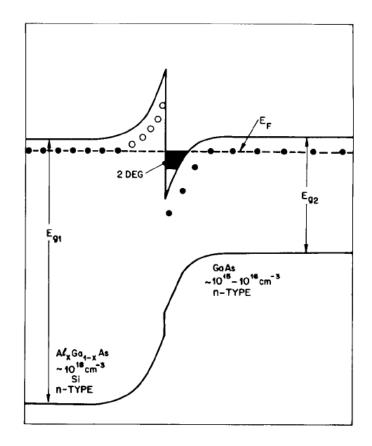
FIGURE B.1 – A two-dimensional electron gas (2DEG) can be created at the interface between two layers with different energy gaps. The 2DEG is fabricated from a GaAS-GaAs<sub>x</sub>Al<sub>1-x</sub> heterostructure grown by Molecular Beam Epitaxy and modulation-doping. Si donors are ionized and the electrostatic field compensates the diffusion current from the low-gap to the wide-gap conductance band : a potential well is established at the interface. From Störmer et al. [141].
