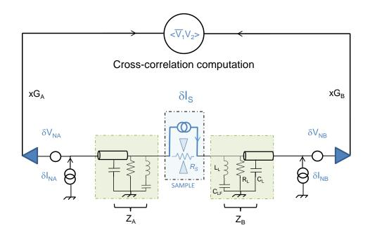
Figure 2.6 – Reduced model for Gain calibration.
