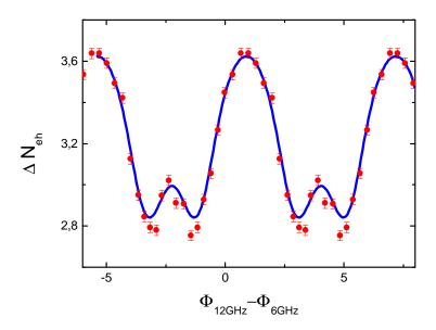
FIGURE 3.9 – Control of Relative Phase between second and first harmonic.  $\nu_0 = 6 \,\text{GHz}$ . Experimental parameters :  $q \sim 1.17$ ,  $\alpha_1 \sim 5.77$  and  $\alpha_2 \sim 2.11$ . This values gives large noise and large contrast. The best fit is based on a full photo-assisted calculation, with a single adjustable parameter : the relative phase induced along the line.
