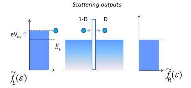
FIGURE 1.2 – Scattering of incoming particles on a localized and energy-independent barrier, with the two possible outputs. D is the transmission probability for a particle, or the amplitude of the transmitted fraction of the wave.
