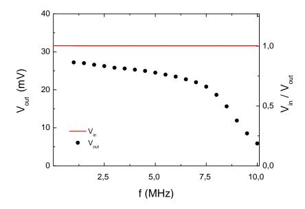
Figure E.2 – Filter calibration with Agilent Acquiris card.
