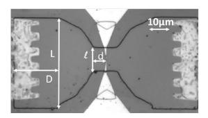
FIGURE B.9 – Electronic microscopy image of mesa and metallic deposition pattern for sample "A". Dimensions are L=  $50 \mu m$ , D =  $25 \mu m$ , l=  $12 \mu m$ , d =  $1 \mu m$ . Adapted from [37].
