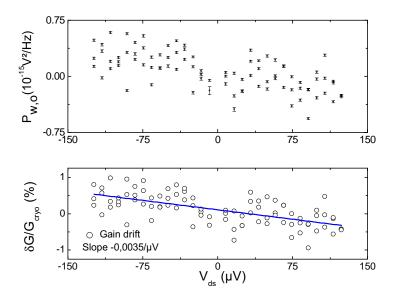
FIGURE C.4 – Gain deviations with bias voltage.
