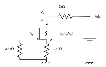
FIGURE F.1 – Set-up for I-V measurement for a self-polarised ATF-34143. Tensions  $V_{ds}$  and  $V_{gs}$  are respectively  $V_d - V_s$  and  $V_g - V_s$ .
