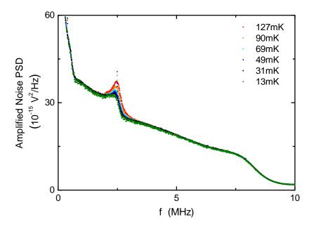
FIGURE 2.13 – Noise Increase with temperature evolution. Auto-correlation spectra from measurement line 1.
