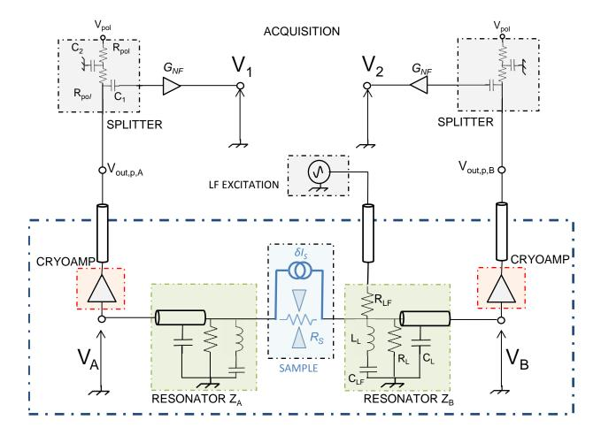
FIGURE 2.1 – Schematic representation of the low-temperature two-channel cross-correlation measurement system. The dotted dark blue box mark the helium-free cryostat. Except for the resistor  $R_{LF}$ , the two channels are entirely identical and labels are not repeated. CRYOAMP and LF-EXCITATION board are detailed in Fig. 2.2 and 2.7.
