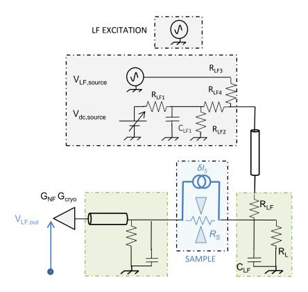
FIGURE 2.7 – Schematic representation of the low-frequency circuit. The DC tension is provided by the DAC auxiliary output of a EG&G 5210 Lock-in. The same Lock-in generates the 497 Hz  $V_{LF,source}$  and extracts  $V_{LF,out}$  from the amplified signal.
