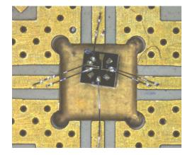
Figure D.3 – Position and bonding of sample "B".
