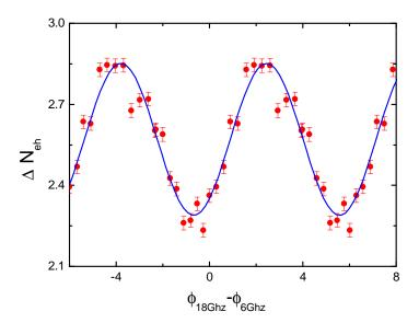
FIGURE 3.8 – Control of Relative Phase between third and first harmonic.  $\nu_0 = 6\,\mathrm{GHz}$ . Experimental parameters : q = 0,  $\alpha_1 \sim 3.97$  and  $\alpha_3 \sim 0.93$ . This set of values gives large noise and large contrast. The best fit is a sine function with a single adjustable parameter : the phase.
