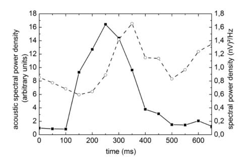
FIGURE 2.21 – Noise level over the band 1–20 kHz measured during a 65 ms time-window at different start time compared to the rotary valve cycle. (Dash line) Acoustic noise power of the pulse tube system. (Solid line) Amplified PSD averaged over a 65 ms time-window at different start time and measured from line B[37].
