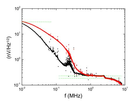
FIGURE 2.23 – Input-referred noise spectrum from 2-HEMT cryoamplifiers, for acquisition line A (red) and B (black). Dashed green lines mark the noise level at the boundaries of the resonance, where no noise current is present.
