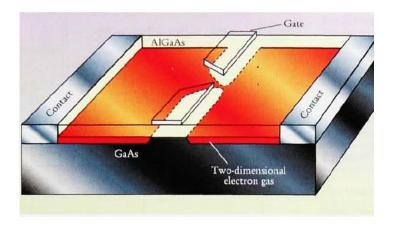
FIGURE B.3 – Density modulation of a 2DEG with a pair of top gates : the split-gate geometry. From the historical review of Van Houten et al.[144].
