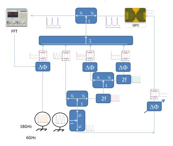
FIGURE 5.3 – RF generation for QST. The Lorentzian pulse(QPC left-contact) with cutoff frequency  $4\nu$  is generated using the compensation system of chapter 3. A phase-locked signal(QPC right-contact) at frequency  $k\nu$  is picked up at the appropriate point in the line (for instance, the case k=1 is represented on the figure). The modulation signal is filtered (pass-band or low-pass) to eliminate undesired harmonics on this side.
