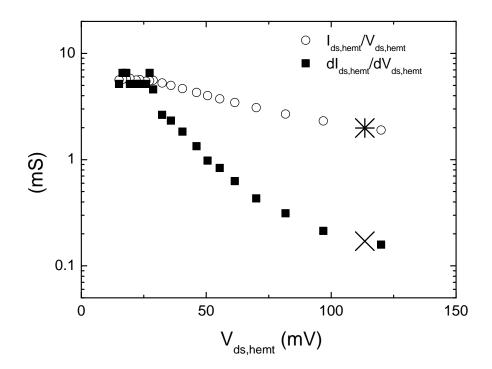
FIGURE F.4 – Black dots represent  $G(I,V_{ds})=I_{ds}/V_{ds}$ , the non-linear conductance of the HEMT channel at 4 K. Black squares represent the constrained differential conductance  $g(I_{ds},V_{ds}(I_{ds}))=dI_{ds}/dV_{ds}$  at 4 K. Fluctuations in square points are a direct consequence of numerical derivation with scarce data points. The polarisation point at which a noise measurement was attempted is marked with a star(cross) shape on the G(g) curve.
