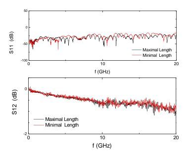
FIGURE A.1 – RF Phase shifters and pulse deformation. Transmission of a DC-18Ghz ARRA inc.  $^{\rm TM}$  model 9425A observed in the two extreme optical path lengths.
