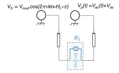
FIGURE 5.1 – Principle of a tomography experiment. A first voltage source is used to apply a pulse  $V_p(t)$  on a contact. A purely harmonic source  $V_S(t)$  is connected to the second contact, with a small peak-peak amplitude  $2V_{mod}$  compared to  $V_p(t)$ . The QPC has a transmission between 0 and 1 in order to generate shot noise.
