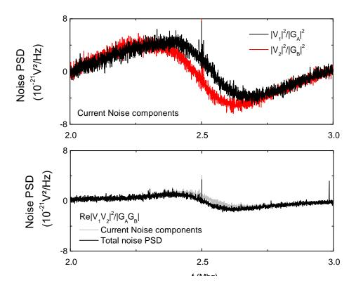
FIGURE 2.26 – Current noise components observed in the equilibrium spectra when D=1 and in input-referred units for the two auto-correlations signal (top part) and the cross-correlated signal (bottom part, black line). The total noise PSD  $|\overline{V_1}V_2|/\overline{G_A}G_B|$  including the thermal noise of all resistors at 35 mK is reproduced (bottom part, grey line). Typically 20000–40000 PSD spectra are averaged together.
