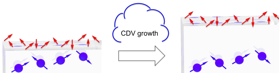
Figure 3.1: Schematic representation for the improvement of the properties of shallow created NV centers, based on the overgrowth of an ultrapure layer of diamond material using plasma vapor deposition.
