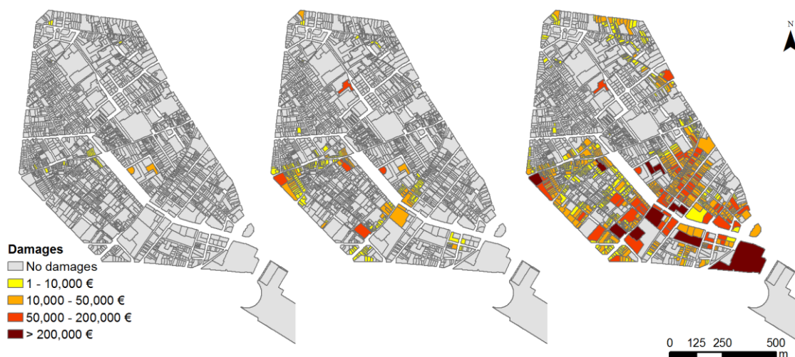
Figure 60: Flood damages in the Raval district for a rain event of return period of 1 year (left), 10 years (centre) and 100 years (right).
