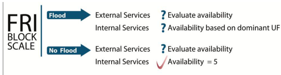
Figure 18: FRI for a block scale with two cases: flooded and no flooded block
