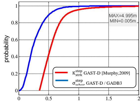
Figure 101: Comparison between observed faulted  $\sigma_{whor}^{step}$  CDF for GAST-D and GAD B3 using ENAC mean probabilities and  $K_{xtrk}^{step}$  generation function from [Murphy et al., 2009] for GAST-D
