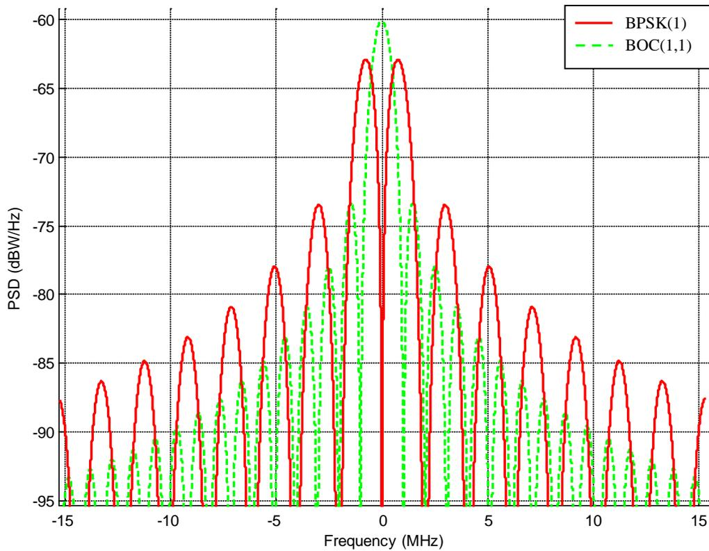
**Figure 4 : BPSK and BOC(1,1) Power Spectrum Density**
