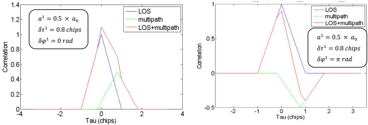
Figure 11 and Figure 12: Correlation function in presence of one multipath for a BPSK(1) signal
