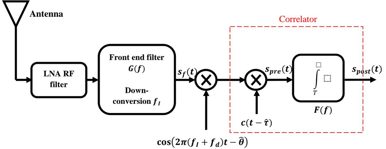
Figure 102: Classical receiver architecture
