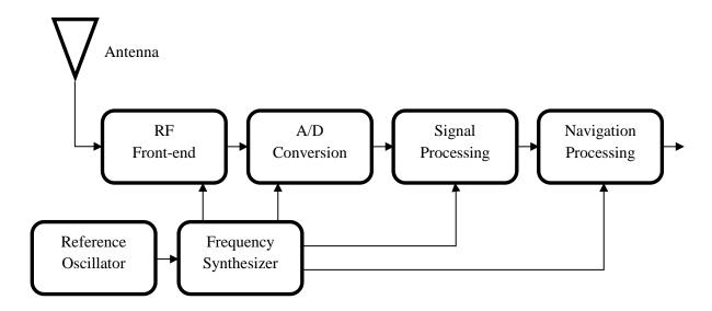
Figure 7: GNSS receiver structure
