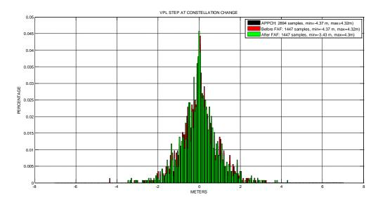
Figure 41: Histogram of VPL steps at constellation change over all simulation runs before and after the FAF in nominal configuration
