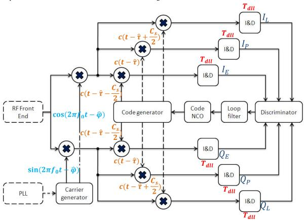
Figure 9: Structure of a classic DLL (with  $T_{dll}$  the correlator integration time)
