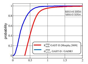
Figure 101: Comparison between observed faulted  $\sigma_{whor}^{step}$  CDF for GAST-D and GAD B3 using ENAC mean probabilities and  $K_{xtrk}^{step}$  generation function from [Murphy et al.,2009] for GAST-D
