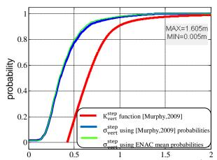
Figure 95: Comparison between observed nominal  $\sigma_{vert}^{step}$  CDF for GAST-D and GAD B3 and  $K_{vert}^{step}$  generation function from [Murphy et al.,2009] for GAST-D
