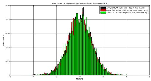
Figure 54: Comparison of the histograms of estimated mean of VPE over all simulation runs before and after the FAF with constellation freezing algorithm
