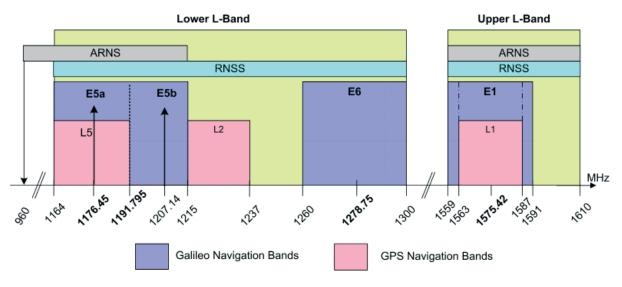
Figure 3: GALILEO frequency plan [GJU, 2010]
