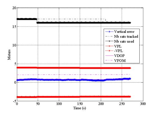
Figure 26: Set 1 - impact of constellation changes on vertical position error (VPE) in meters, VPL, VDOP and VFOM for nominal configuration
