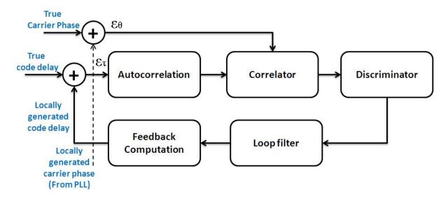
Figure 21: structure of the simulated DLL
