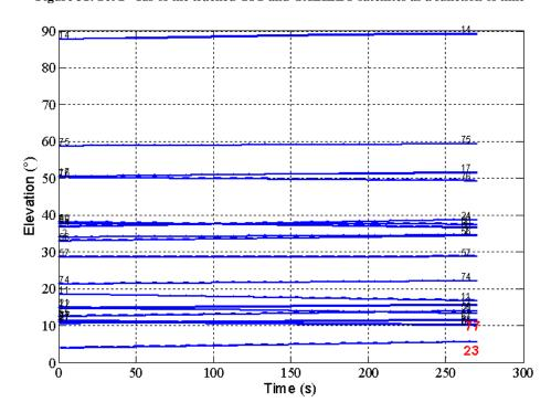
Figure 32: Set 2 - Elevation angle of GPS and GALILEO satellites as a function of time
