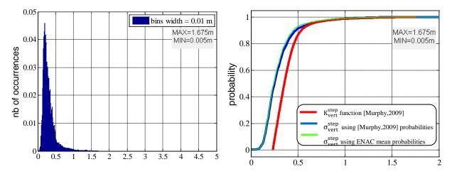
Figure 82: Observed nominal  $\sigma_{vert}^{step}$  distribution for GAST-C and GAD B3 using ENAC mean probabilities
