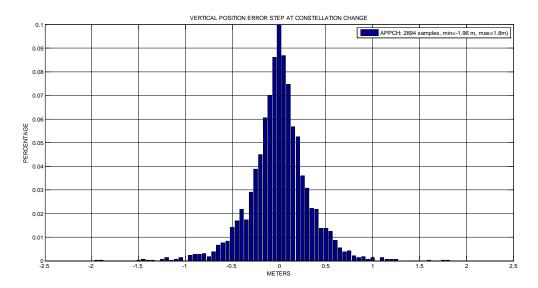
Figure 36: Histogram of VPE steps at constellation change over all simulation runs for the complete approaches in nominal configuration
