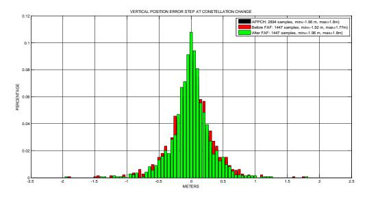
Figure 40: Comparison of the histograms of VPE steps at constellation change over all simulation runs before and after the FAF in nominal configuration
