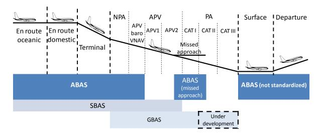
Figure 1: Phases of flight and GNSS augmentations [MONTLOIN, 2011]
