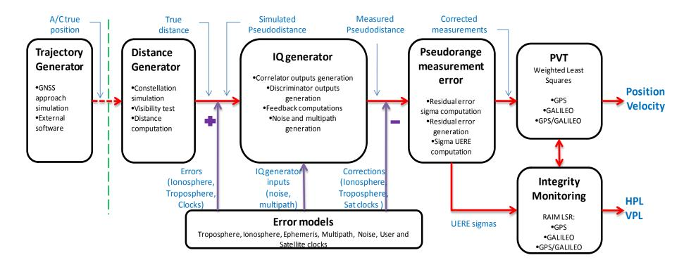
Figure 16: Receiver Simulator architecture
