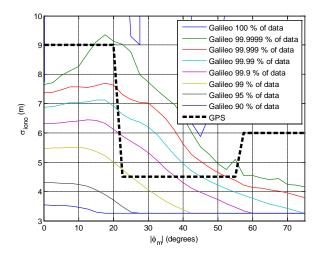
Figure 15: GALILEO and GPS ionospheric residual error model [SALOS, 2010]
