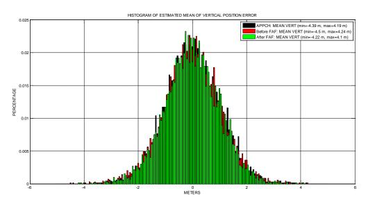
Figure 38: Comparison of the histograms of the estimated mean of VPE over all simulation runs before and after the FAF in nominal configuration
