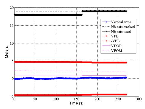
Figure 30: Set 2 - impact of constellation changes on Vertical Position Error (VPE) in meters, VPL, VDOP and VFOM for nominal configuration
