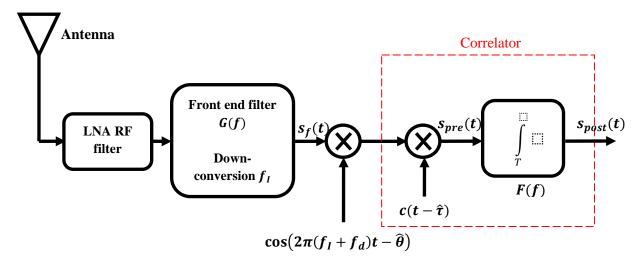
Figure 102: Classical receiver architecture
