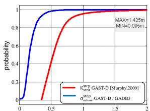
Figure 97: Comparison between observed nominal  $\sigma_{whor}^{step}$  CDF for GAST-D and GAD B3 using ENAC mean probabilities and  $K_{xtrk}^{step}$  generation function from [Murphy et al.,2009] for GAST-D
