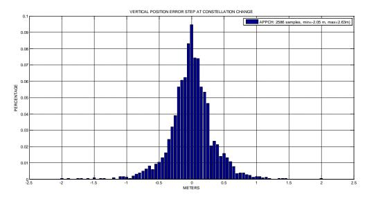
Figure 52: Histogram of VPE steps at constellation change over all simulation runs for the complete approaches
