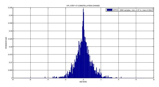
Figure 37: Histogram of VPL steps at constellation change over all simulation runs for the complete approaches in nominal configuration
