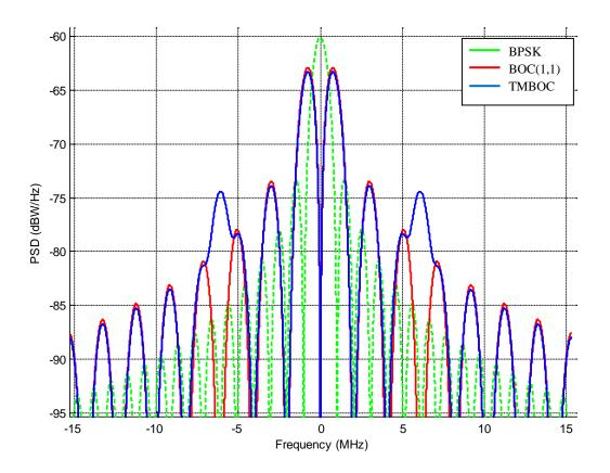
Figure 6: MBOC Power Spectral Density
