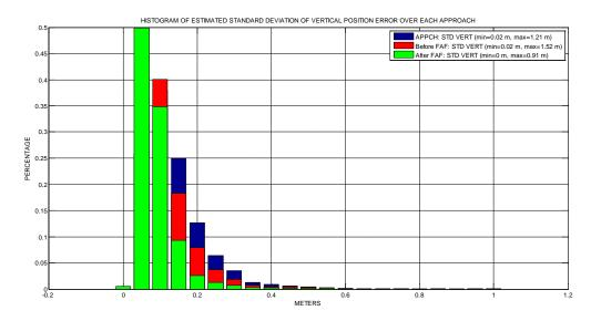
Figure 39: Comparison of the histograms of estimated standard deviation of VPE over all simulation runs before and after the FAF in nominal configuration
