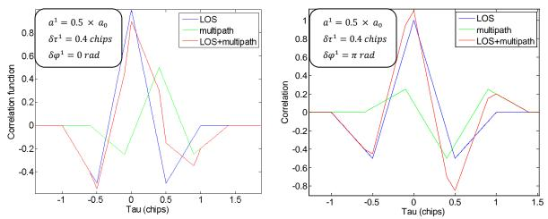
Figure 13 and Figure 14: Correlation function in presence of one multipath for a BOC(1,1) signal
