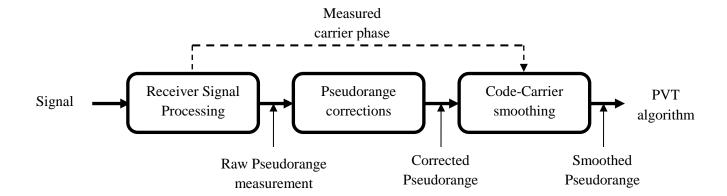
Figure 10: Elaboration of GNSS measurements
