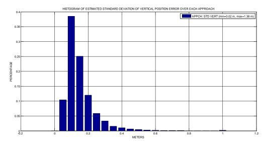
Figure 51: Histogram of estimated std of VPE over all simulation runs for the complete approaches
