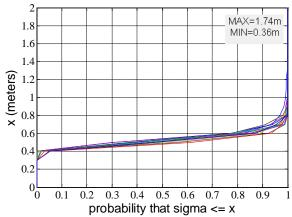
Figure 65: observed  $\sigma_{vert}$  histograms superimposed for all airports for GAST-C and GAD B3 using DO-245A probabilities
