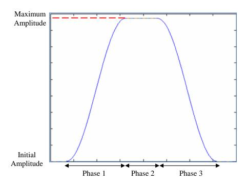
Figure 20: Raised Cosine for attitude angles simulation
