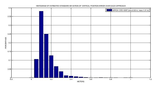
Figure 35: Histogram of estimated standard deviation of VPE over all simulation runs for the complete approaches in nominal configuration
