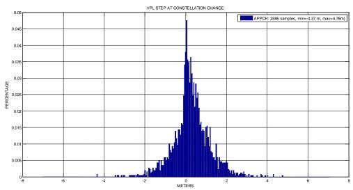
Figure 53: Histogram of VPL steps at constellation change over all simulation runs for the complete approaches
