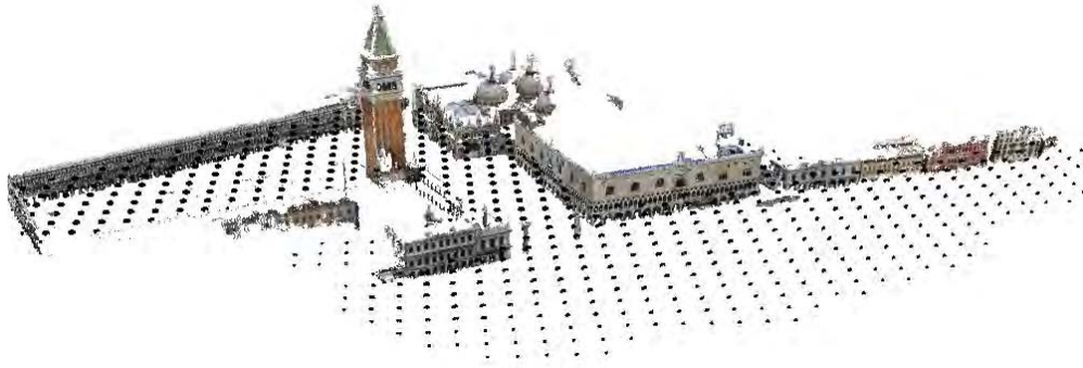
Figure 4.4: Example sampled viewpoints. Camera positions are sampled on the ground plane on a regular 100\times 100 grid. 24 camera orientations are used for each viewpoint. Cameras not viewing any portion of the 3D model are discarded. This procedure results in about 45,000 valid views for the depicted 3D model.
