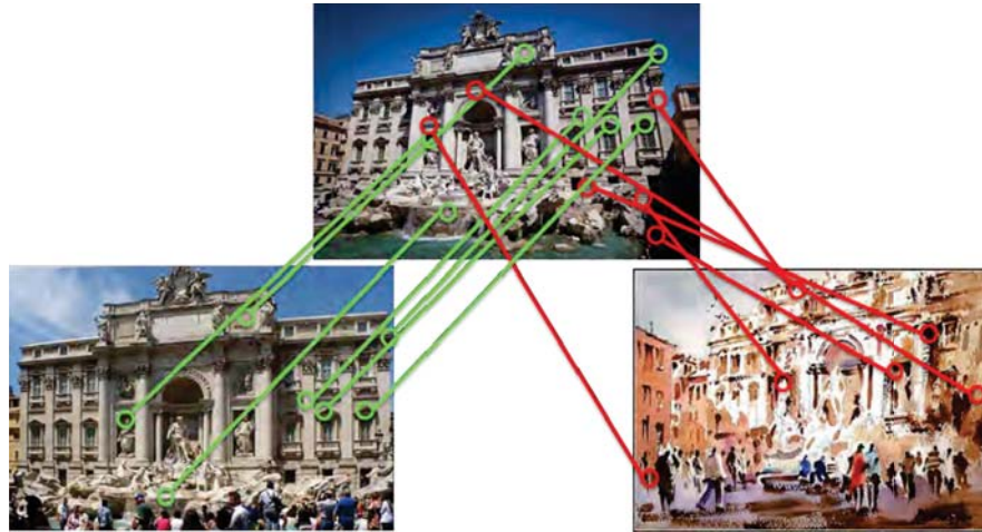
Figure 1.5: Matching local features, such as SIFT [121] often works well for two similar photographs (left), but fails between two very different images such as a photograph and a watercolor (right). This figure shows the most confident SIFT matches between the top image and the two bottom images in terms of the first to second nearest neighbor ratio [121].
