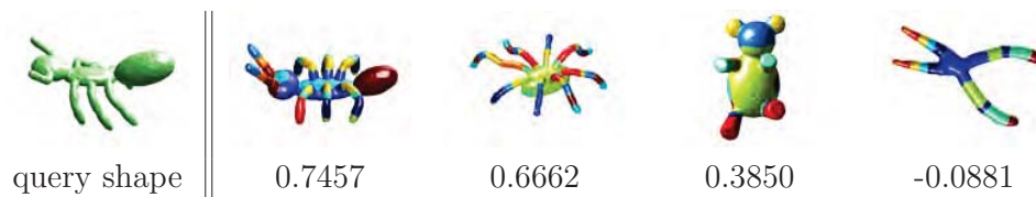
Figure 3.15: Shape segmentation applied to shape retrieval on the SHREC 2010 dataset [116]. The four columns on the right show representatives of four shape classes. For each shape class a Gaussian mixture distribution was computed as outlined in Section 3.5. The resulting segmentations are color encoded. The log-likelihood of the query shape (leftmost column) with respect to these distributions is displayed below each class.
