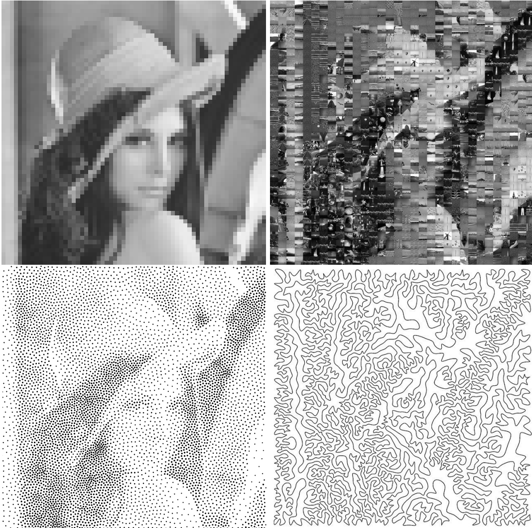
Figure 3.1: “Lena” and three large error approximations. Top left: pixellized 64 \times 64 sub-sampling. Top right: photomosaics as pioneered in [123] (credit: [1]). Bottom left: stippling (6000 stipples). Bottom right: TSP art (credit Seb Perez-Duarte via Flickr).
