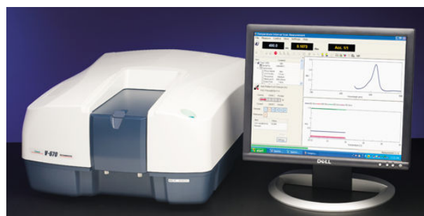
Figure 2.22: V-670 Jasco spectrophotometer and relative software.
