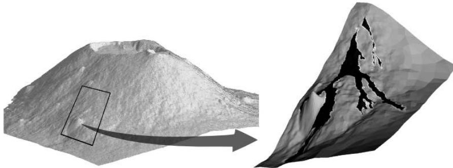
FIGURE 5.7 – Digital elevation model of the Piton de la Fournaise volcano in 2008, with a 5 meter horizontal resolution (left). Zoom with the observed arrested flow contours (right).
