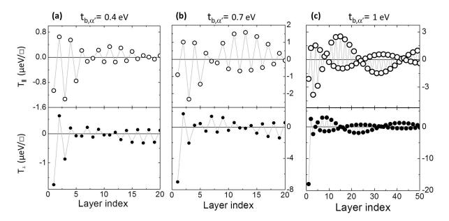
Figure III.24 – Computed spatial distributions of the in-plane  $(T_{\parallel})$  and out-of-plane  $(T_{\perp})$  components of the torque in  $\mu eV$  per unit of surface  $\Box$  for a 3-D FI/B/FI junction with  $\theta = \pi/2$ , V= -0.1V,  $\epsilon_0 = 1.5 eV$ ,  $\Delta_A = 0.5 eV$  and  $\Delta_B = 0.25 eV$  in both FI leads. The hopping parameter at the barrier interfaces (coupling) is  $t_{b,\alpha'} = t_{a,\alpha} =$  (a) 0.4 eV. (b) 0.7 eV. (c) 1 eV.
