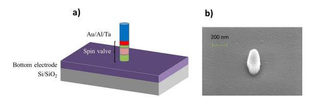
Figure C.6 – Fifth step: **a**) Reactive-ion etching (RIE) of the 150 nm of Ta. The Pt protects the nanopillars from etching. The end of the etching process is checked by laser monitoring. Subsequent ion beam etching (IBE) down to the bottom electrode is performed to remove the rest of the layers. Secondary ion mass spectrometry is used to know when to stop etching. **b**) Scanning electron microscope (SEM) image of the bare nanopillar (around 150 nm wide).
