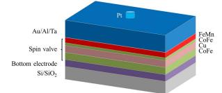
Figure C.5 – Fourth step: resist lift-off to leave only the Pt layer on the ellipses and circles covering the stack.
