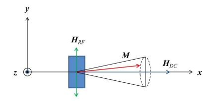
Figure IV.4 – Schematic illustration of the FMR measurement configuration: the static DC field is applied in the plane of the sample along the  $\mathbf{x}$  direction; the RF field is applied in the plane of the sample perpendicular to the DC field.
