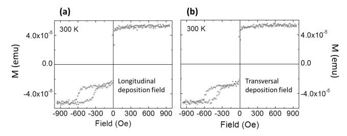
Figure IV.15 – (a) Hysteresis loop measured along the longitudinal direction at 300 K for a  $Si/SiO_2/NiFe(8)/Cu(3)/NiFe(3)/IrMn(7)/Al(2)$  stack annealed 1 hour under longitudinal field at 300°C. (b) Hysteresis loop measured along the transverse direction at 300 K for a similar stack annealed 1 hour under transverse field at 300°C.
