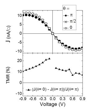
Figure III.12 – Calculated voltage dependence of the charge current density J in nA by unit of surface  $\Box$  for three different angles  $\theta$  (top) and TMR (bottom) in a 3-D AF/B/AF tunnel junction with  $\Delta = 0.5$  eV and  $\epsilon_0 = 1.5$  eV in both AF leads.
