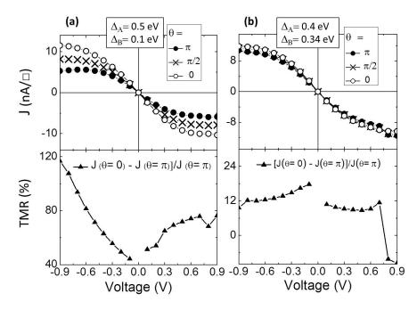
Figure III.25 – Calculated voltage dependence of the charge current density I in nA by unit of surface  $\Box$  for three different angles  $\theta$  (top) and TMR (bottom) in a 3-D FI/B/FI tunnel junction with (a)  $\Delta_A = 0.5$  eV;  $\Delta_B = 0.25$  eV. (b)  $\Delta_A = 0.4$  eV;  $\Delta_B = 0.34$  eV.
