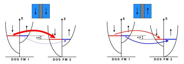
Figure I.4 – Schematic explanation of the TMR effect in terms of the spin-split DOS of two identical F leads for parallel (left) and antiparallel (right) states. The resistance in the parallel state is lower since the DOS at the Fermi level for majority down electrons at both leads is high. The Fermi levels at the left and right leads are shifted with respect to each other by an energy eU when a voltage U is applied across the structure.
