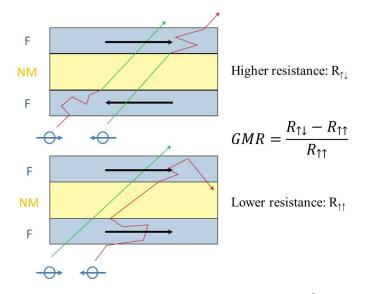
Figure I.2 – Schematic illustration of GMR adapted from Ref. [Chappert et al., 2007] and definiton of the GMR ratio.
