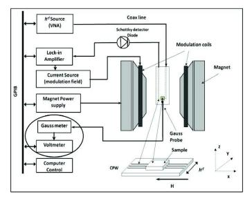
Figure IV.9 – FMR measurement setup scheme
