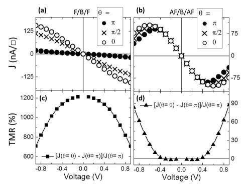
Figure III.11 – Calculated voltage dependence of the charge current density J in nA per unit of surface  $\Box$  for three different angles  $\theta$  (top) and TMR (bottom) in (a)-(c) a 3-D F/B/F tunnel junction with  $\Delta = 0.75$  eV in both F leads and in (b)-(d) a 3-D AF/B/AF tunnel junction with  $\Delta = 1$  eV and  $\epsilon_0 = 2$  eV in both AF leads.
