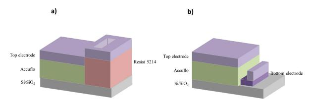
Figure C.11 – **a)** Twelfth step: electron-beam evaporation of the top electrode: Cr(10)/Al(200)/Ti(5)/Au(100). **b)** Thirteenth step. Resist lift-off.
