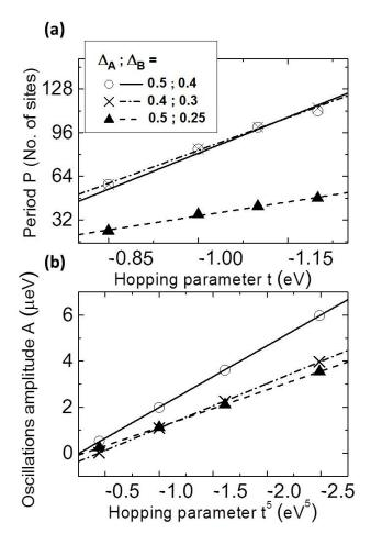
Figure III.17 – (a) Dependence on the hopping parameter t of the in-plane torque component waves period P for  $\theta = \pi/2$  and V= -0.1V. (b) Corresponding dependence with  $t^5$  of the torque waves amplitude. The three FI leads of (a) and (b) have  $\Delta_A$  and  $\Delta_B$  given in eV in the caption of (a). The lines are linear fit to the data.
