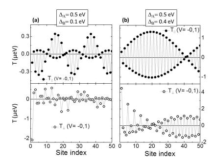
Figure III.15 – Computed spatial distributions of the in-plane  $(T_{\parallel})$  and out-of-plane  $(T_{\perp})$  components of the torque in  $\mu eV$  for a 1-D FI/B/FI junction with  $\theta = \pi/2$ , V= -0.1V,  $\epsilon_0 = 1.5 eV$  and (a)  $\Delta_A = 0.5 eV$ ;  $\Delta_B = 0.1 eV$  ( $\delta = 0.4 eV$ ). (b)  $\Delta_A = 0.5 eV$ ;  $\Delta_B = 0.4 eV$  ( $\delta = 0.1 eV$ ).
