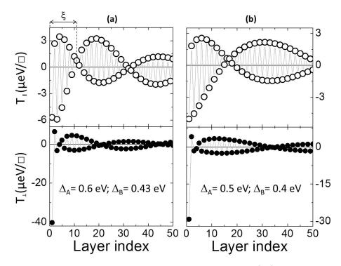
Figure III.20 – Computed spatial distributions of the in-plane  $(T_{\parallel})$  and out-of-plane  $(T_{\perp})$  components of the torque in  $\mu eV$  per unit of surface  $\Box$  for a 3-D FI/B/FI junction with  $\theta = \pi/2$ , V= -0.1V,  $\epsilon_0 = 1.5 eV$  and (a)  $\Delta_A = 0.6 eV$ ;  $\Delta_B = 0.43 eV$  ( $\delta = 0.17 eV$ ). (b)  $\Delta_A = 0.5 eV$ ;  $\Delta_B = 0.4 eV$  ( $\delta = 0.1 eV$ ).
