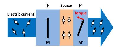
Figure I.6 – Conducting electrons flowing through the first thin F layer get spin polarized along the magnetization  $\mathbf{M}$ . If magnetizations  $\mathbf{M}$  and  $\mathbf{M}$ ' are not collinear, the spin orientation of the polarized electrons is modified again when traversing the second F' thin layer. This last change of spin angular momentum of conducting electrons implies a torque exerted on the magnetization  $\mathbf{M}$  hence the term spin transfer torque.
