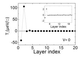
Figure III.7 – Spatial distribution of the out-of-plane torque in  $\mu$ eV per unit of surface  $\Box$  at zero bias (RKKY interaction) for a 3-D AF/B/AF junction with  $\theta = \pi/2$ , V= -0.1V,  $\epsilon_0 = 1.5$ eV and  $\Delta = 0.5$  eV in both AF leads. The inset is a zoom of the torque from the third layer.
