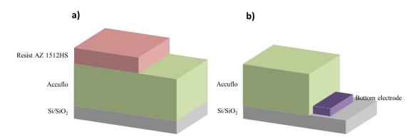
Figure C.8 – **a**) Eighth step: spin coating of the sample with Accuflo polymer to insulate the bottom and top electrodes. Spin coating with AZ 1512HS resist, ultra violet lithography and resist development to custom the insulating zone near the nanopillar. **b**) Ninth step. RIE of the insulator. The end of the etching process is checked by laser monitoring.
