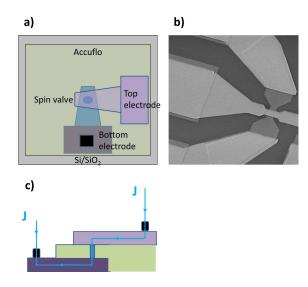
Figure C.12 – **a**) Schematic top view of the magnetic nanostructure. **b**) SEM image of the patterned nanostructure showing the top and bottom contacts. **c**) Schematic illustration of the current flow through the nanostructure. The nanopillar is encapsulated in the Accuflo insulator and contacted by the electrodes.
