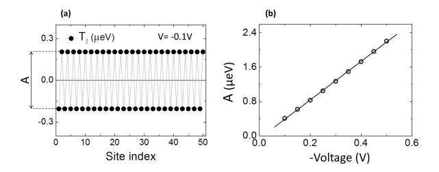
Figure III.4 – (a) Definition of the amplitude A (in  $\mu eV$ ) of the in-plane torque in a 1-D AF/B/AF junction with  $\theta = \pi/2$ , V= -0.1V,  $\epsilon_0 = 1.5$  eV and  $\Delta = 0.5$ eV. (b) Voltage dependence of A in the same system. The line is a linear fit to the data.
