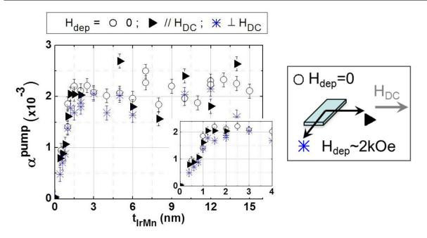
Figure IV.13 – Dependence with  $t_{\rm IrMn}$  of the IrMn contribution, via spin pumping, to the NiFe magnetization damping ( $\alpha^{\rm pump}$ ) for Si/SiO<sub>2</sub>//NiFe(8)/Cu(3)/IrMn( $t_{\rm IrMn}$ )/Al(2) (nm) stacks with various IrMn thicknesses ( $t_{\rm IrMn}$ ) and for various directions of magnetic field applied during deposition ( $H_{\rm dep}$ ). The inset is a zoom of the low thicknesses region.
