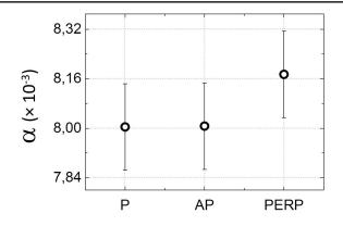
Figure IV.14 – Total damping parameter  $\alpha$  for three Si/SiO<sub>2</sub>//NiFe(8)/Cu(3)/NiFe(3)/IrMn(7)/Al(2) (nm) stacks annealed 1 hour at 300° C under applied magnetic field along three directions: transversal to the sample and parallel to the DC field, (P), transversal to the sample and antiparallel to the DC field, (AP), and longitudinal to the sample and perpendicular to the DC field  $\mathbf{H}_{DC}$ , (PERP).
