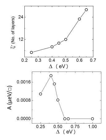
Figure III.27 – Variation of the wave length scale  $\xi'$  and the amplitude A with the spin splitting  $\Delta$  in a 3-D AF/B/AF junction of compensated layers with  $\theta = \pi/2$ ,  $\epsilon_0 = 1.5$ eV and V= -0.1 V.
