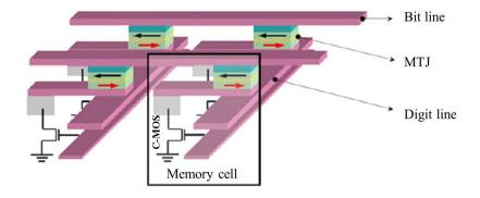
Figure I.5 – Basic cross point architecture of MRAM adapted from Ref. [Prejbeanu et al., 2013]. The working principle is explained in the text.
