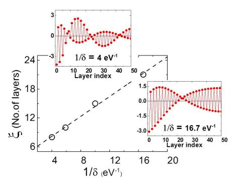
Figure III.22 – For four 3-D FI leads,  $1/\delta$  dependence of the torque characteristic length  $(\xi)$  for  $\theta = \pi/2$  and V= -0.1V. Upper(Lower) inset: spatial distribution (in  $\mu$ eV per unit area) of the in-plane torque wave for  $1/\delta = 4 \text{ eV}^{-1}$  ( $1/\delta = 16.7 \text{ eV}^{-1}$ ). The dashed line is a linear fit to the data.
