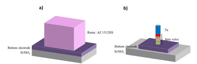
Figure C.7 – **a**) Sixth step: spin coating of the sample with AZ 1512HS resist, ultra violet lithography and resist development to pattern the bottom electrode. **b**) Seventh step. IBE of the bottom electrode. Resist lift off by RIE using a  $O_2$  plasma to remove the resist burnt during the IBE, acetone and ultra sounds.
