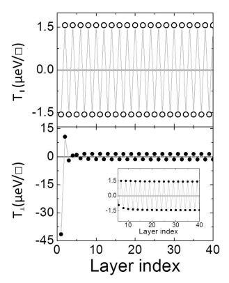
Figure III.6 – Computed spatial distributions of the total in-plane  $(T_{\parallel})$  and out-of-plane  $(T_{\perp})$  components of the torque in  $\mu$ eV per unit of surface  $\Box$  for a 3-D AF/B/AF junction with  $\theta = \pi/2$ , V= -0.1V,  $\epsilon_0 = 1.5$ eV and  $\Delta = 0.5$  eV in both AF leads. The inset is a zoom of the out-of-plane component from the sixth layer to stress its staggered character.
