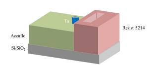
Figure C.10 – Eleventh step: spin coating of the sample with AZ 5214 resist. Ultra-violet lithography and development to custom the shape of the top electrode.
