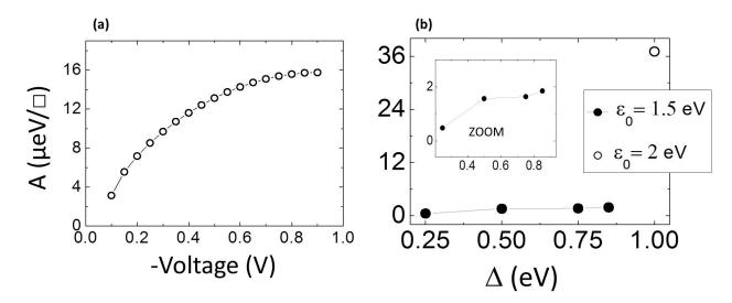
Figure III.9 – (a) Dependence of the in-plane torque amplitude A in  $\mu eV$  per unit of surface  $\Box$  on the applied voltage for a 3-D AF/B/AF junction with  $\theta = \pi/2$  and  $\Delta = 0.5$  eV. (b) Dependence of the in-plane torque amplitude A on the spin splitting  $\Delta$  for the same junction at V= -0.1V. The inset is a zoom for the low values of the amplitude.
