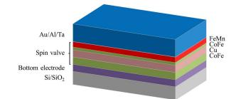
Figure C.3 – First step: annealing of the stack for 30 minutes at  $250^{\circ}$ C under in plane magnetic field in a  $10^{-6}$  mbar vacuum chamber.
