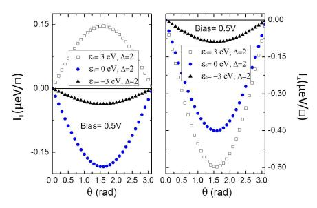
Figure III.5 – (Left) Angular dependence of the in-plane spin current density component for three different 3-D AF/B/AF MTJ with a bias of 0.5V and a barrier height  $U_B$  of 9 eV. (Right) Idem for the out-of-plane component.
