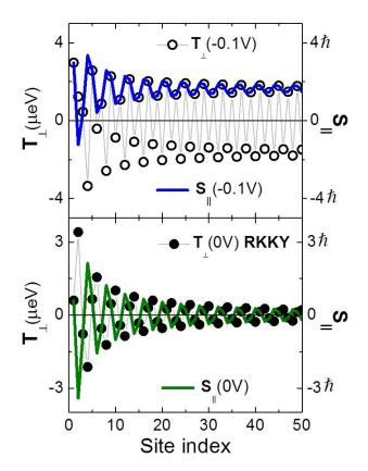
Figure III.3 – Computed spatial distribution of the total out-of-plane torque  $T_{\perp}$  and the total in-plane spin density  $S_{\parallel}$  for a 1-D F/B/AF junction with  $\theta = \pi/2$  at -0.1V and 0V (RKKY interaction) with  $\Delta = 0.5$  eV for both F and AF leads. The blue and green thick lines representing respectively the in-plane spin densities at -0.1V (top) and 0V (bottom) refer to the right-hand ordinate.
