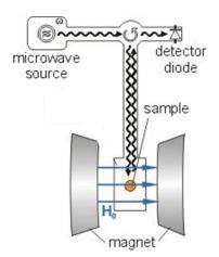
Figure IV.3 – Scheme of the FMR measurement setup
