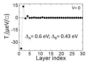
Figure III.21 – Spatial distribution of the out-of-plane torque in  $\mu$ eV per unit of surface  $\Box$  at zero bias (RKKY interaction) for a 3-D FI/B/FI junction with  $\theta = \pi/2$ , V= -0.1V,  $\epsilon_0 = 1.5$  eV,  $\Delta_A = 0.6$  eV and  $\Delta_B = 0.43$  eV ( $\delta = 0.17$  eV).
