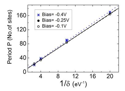
Figure III.18 – For different 1-D FI/B/FI MTJ,  $1/\delta$  dependence of the in-plane torque component period P for  $\theta = \pi/2$  and three different applied bias. The dash black, solid black and dot blue lines are linear fits to the data corresponding to -0.1V, -0.25V and -0.4V respectively.
