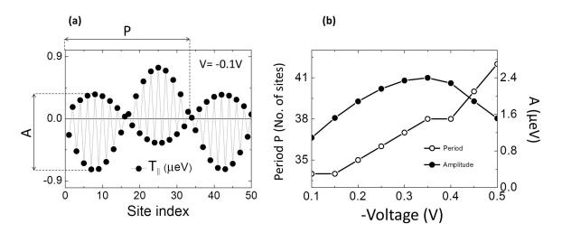
Figure III.14 – (a) Definition of the amplitude A (in  $\mu$ eV) and the period P (in number of layers) of the in-plane torque in a 1-D FI/B/FI junction with  $\theta = \pi/2$ , V= -0.1V,  $\epsilon_0 =$ 1.5 eV,  $\Delta_A = 0.5$  eV and  $\Delta_B = 0.25$  eV. (b) Voltage dependence of P (open circles referred to the left hand ordinate) and A (solid circles referred to the right hand ordinate) in the same system.
