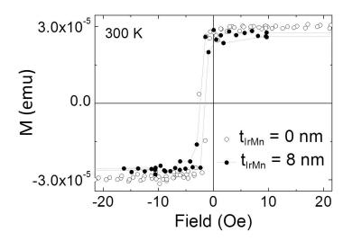
Figure IV.8 – Hysteresis loops at 300K for two Si/SiO<sub>2</sub>/NiFe(8)/Cu(3)/IrMn( $t_{\rm IrMn}$ )/Al(2) stacks with  $t_{\rm IrMn} = 0$  (open circles) and 8 nm (solid circles).
