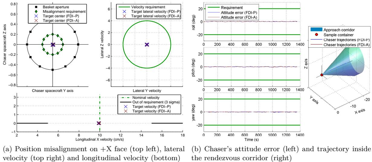
Figure 3.14 – Capture position requirements and GNC performances for fault Case 2
