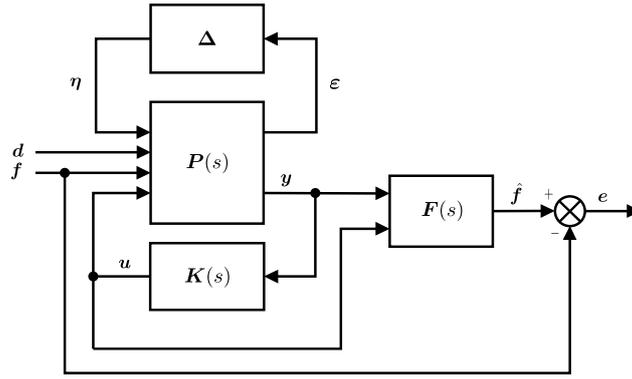
Figure 1.7 – The  $H_\infty$  fault estimation problem
