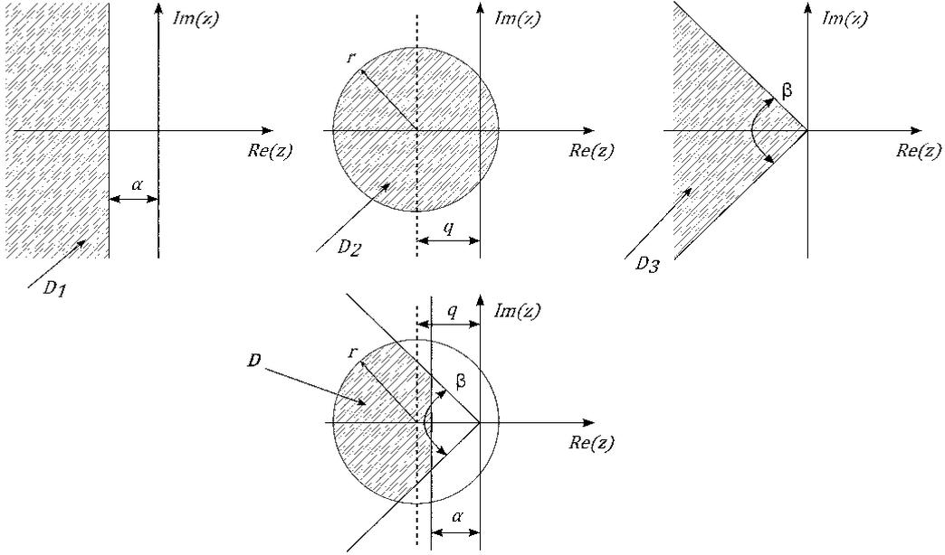
Figure 4.4 – LMI Region  $\mathcal{D}(\alpha, q, r, \beta) = \mathcal{D}_1 \cap \mathcal{D}_2 \cap \mathcal{D}_3$
