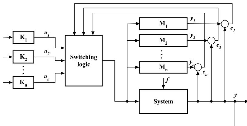
Figure 1.19 – Multiple model switching and tuning scheme
