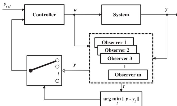
Figure 1.20 – Bank of observers for sensor faults
