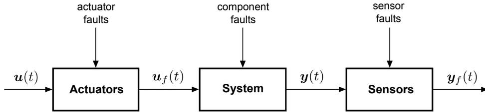
Figure 1.2 – Open-loop system with different types of faults
