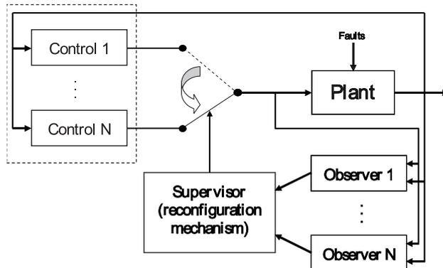
Figure 1.26 – The structure of the supervisory FTC architecture
