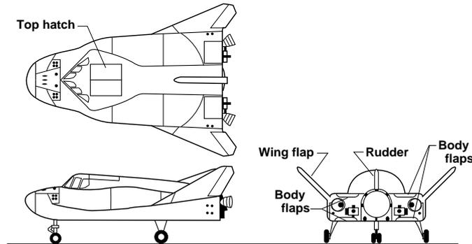
Figure 1.6 – The HL-20 RLV vehicle, ©1998 NASA
