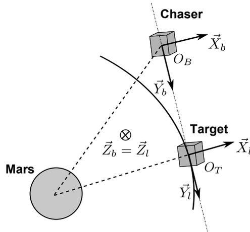
Figure 2.18 – Chaser attitude target pointing mode
