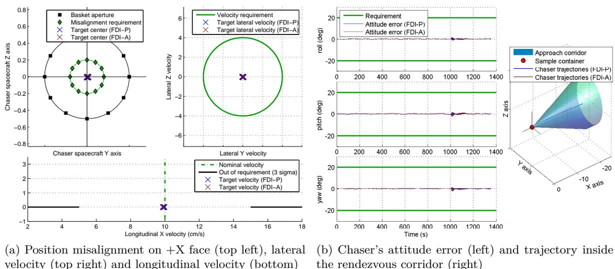
Figure 3.16 – Capture position requirements and GNC performances for fault Case 3
