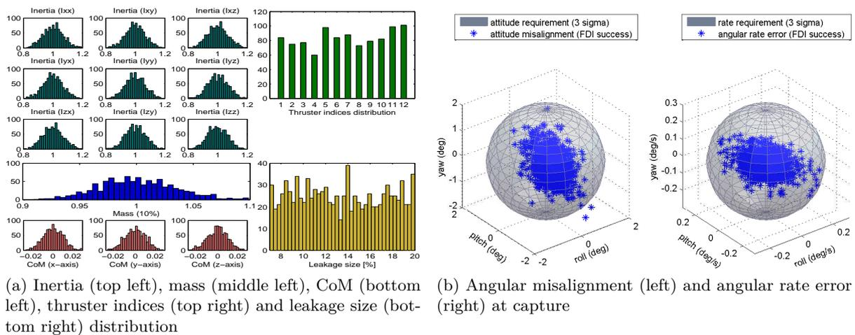
(a) Inertia (top left), mass (middle left), CoM (bottom left), thruster indices (top right) and leakage size (bottom right) distribution (b) Angular misalignment (left) and angular rate error (right) at capture
