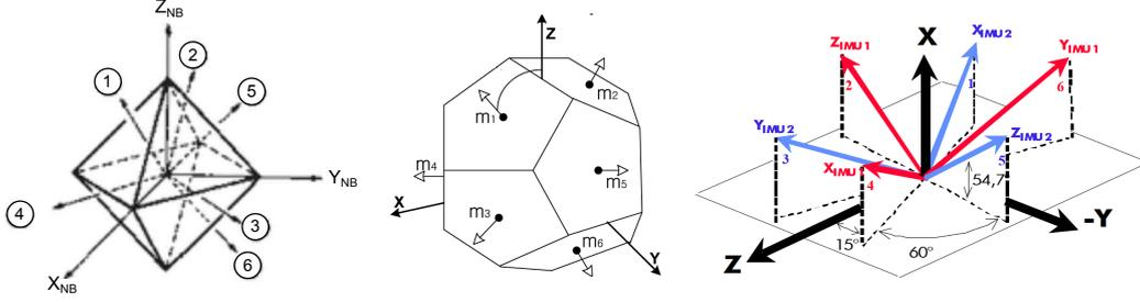
Figure 1.3 – The octahedron (left), the dodecahedron (centre) and the dedicated pyramid (right) configurations [135]
