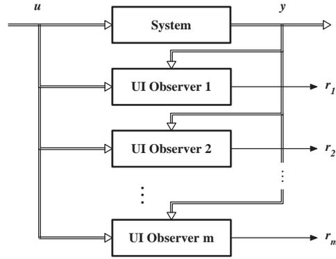
Figure 1.16 – General structure of the UIO scheme
