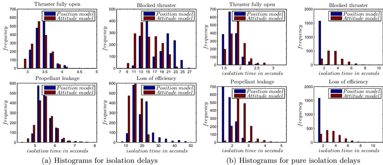
Figure 3.12 – Histograms for isolation and pure isolation delays
