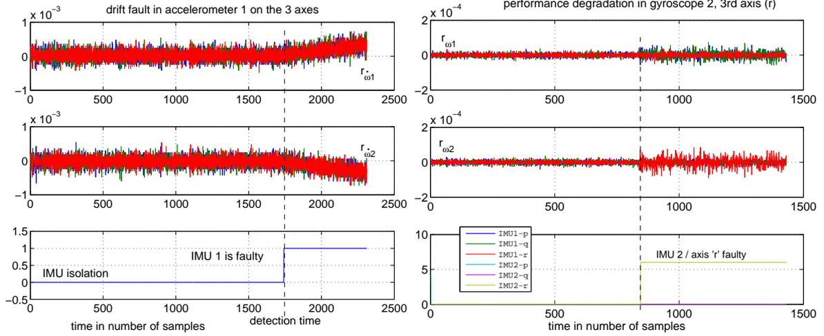
Figure 2.15 – Sensor drift in the 1<sup>st</sup> accelerometer (left) and performance degradation of the 2<sup>nd</sup> gyro (right)
