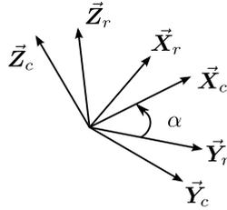
Figure 2.9 – Geometrical interpretation of zeroing the off-diagonal elements of  $\mathbf{A}_\epsilon$ .
