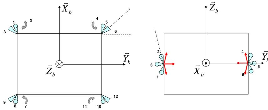
Figure 4.1 – Thruster configuration of the chaser spacecraft
