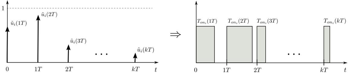
Figure 2.13 – Scaled ON-times versus real thruster firing durations
