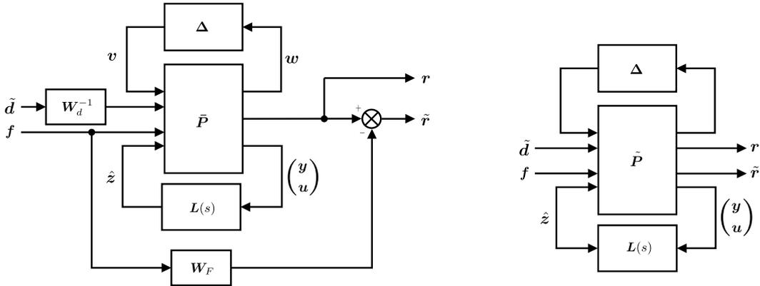
Figure 1.9 – The quasi standard setup for the design of a robust fault detection filter
