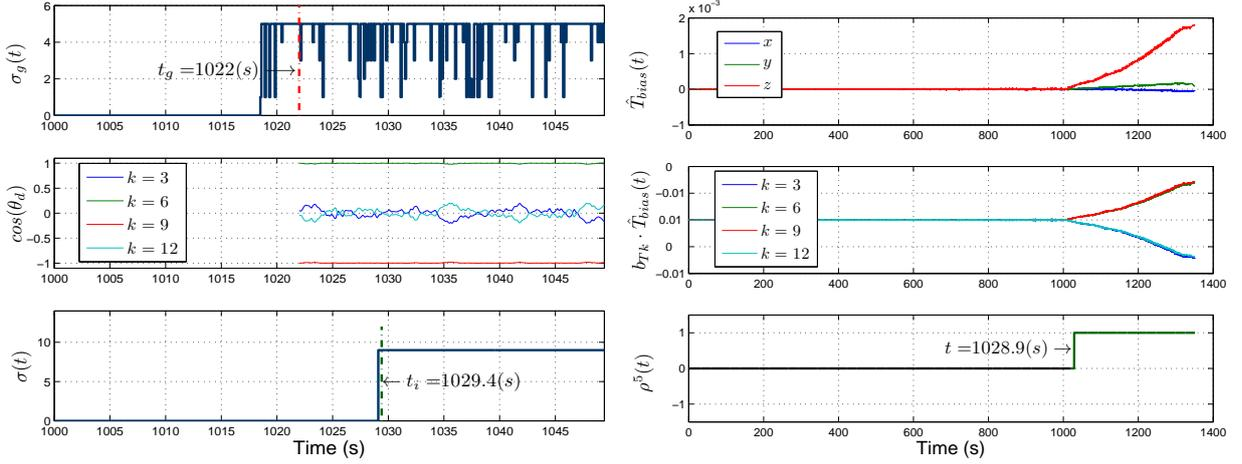
(a) Faulty thruster group isolation (top), directional cosines within the isolated group (middle) and isolation rule signal (bottom) (b) Torque bias direction estimates (top), bias directions relative to torque directions within the isolated group (middle) and the Wald's test behaviour (bottom)
