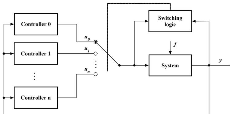
Figure 1.18 – Structured scheme of the multiple-model approach
