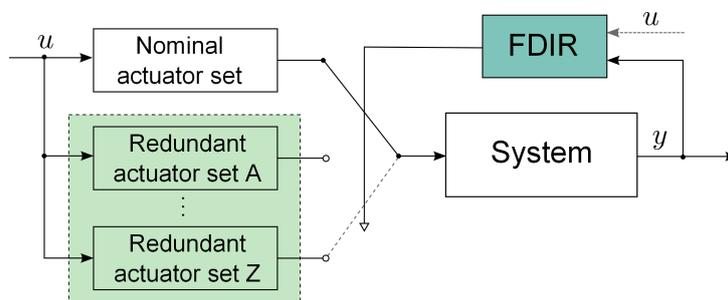
Figure 3.1 – “Half satellite” strategy for thruster faults
