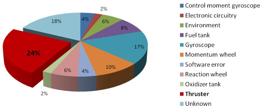
Figure 1 – Distribution of AOCS component faults
