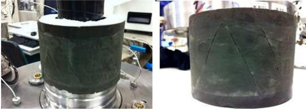
Fig. 6. COx claystone at the end of the test T1.
