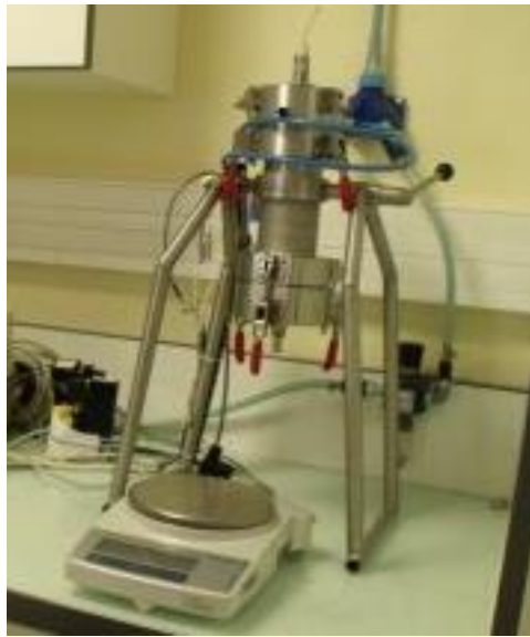
Figure 5-17 Cellule de filtration compression.
