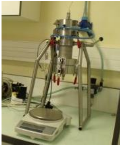
Figure 5-17 Cellule de filtration compression.
