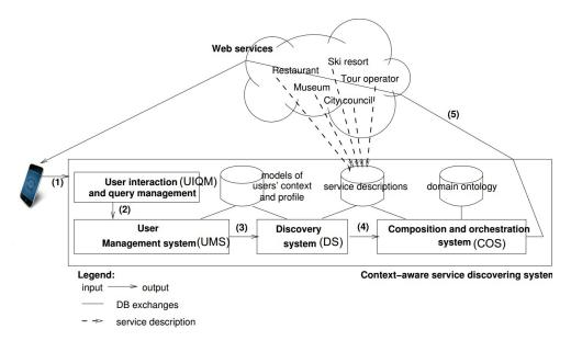
Figure 1.1: Architecture of a system for discovering, execution and composition of services for mobile users [LLK+11]
