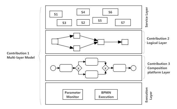
Figure 1.2: Multi-layer for service composition and execution system
