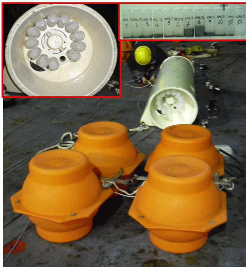
Fig.2.3 Sediment trap device, as well as the collecting cups after the CASCADE campaign Same equipments were used in the HERMES deployment.
