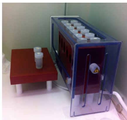
Fig.2.7 Hot plate and heating device for teflon beakers in the clean room
