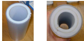
Figure 5: Test duct with melamine foam: (left) \delta = 10 mm and (right) \delta = 20 mm.
