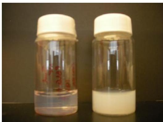
**Figure 3:** PBLG<sub>25k</sub>-*b*-PGlu<sub>2k</sub> nanoparticle suspensions prepared from the novel nanoprecipitation method: left: in presence of sodium hydroxide; right: in absence of sodium hydroxide
