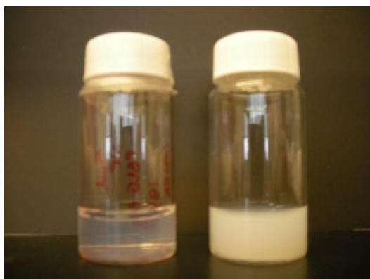
Figure 3: PBLG 25k - b -PGlu 2k nanoparticle suspensions prepared from the novel nanoprecipitation method: left: in presence of sodium hydroxide; right: in absence of sodium hydroxide
