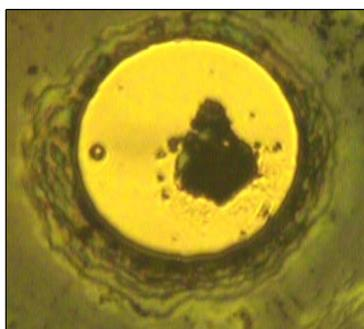
Figure 4.2: Picture of a Fe sample completely embedded in a KCl pressure transmitting. The ruby pressure gauge is also visible in the picture near the gasket-KCl interface (circle on the left).
