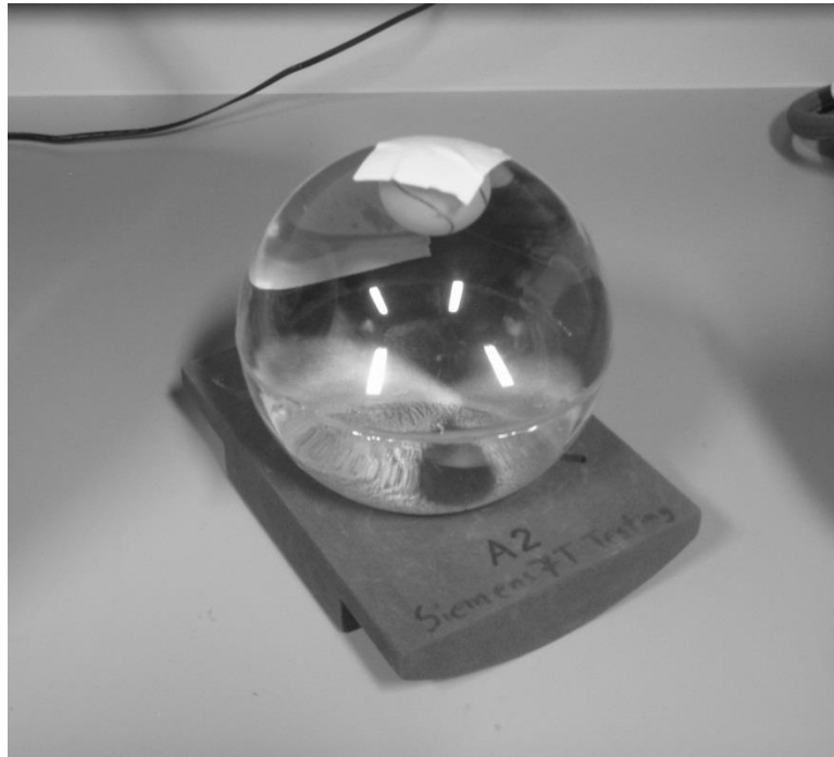
Figure 3.6: Picture of one of the MRI phantoms made (16 cm diameter).
