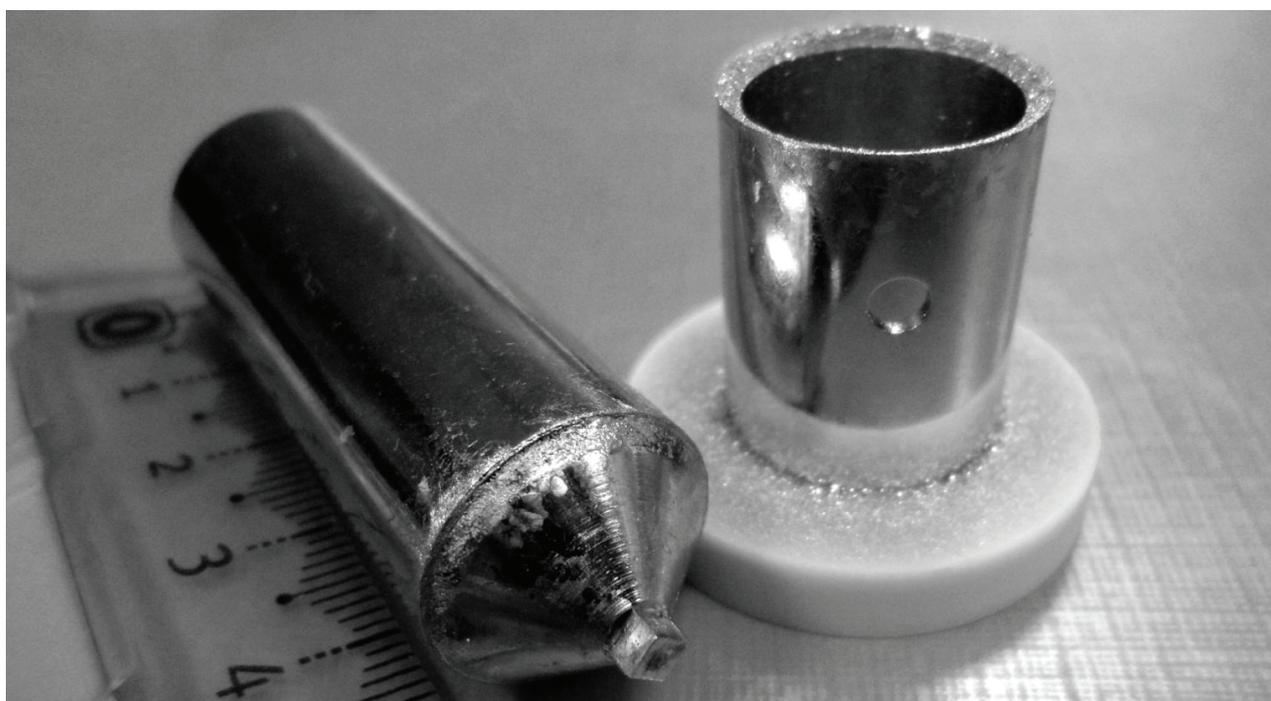
Figure II.1. Ir crucible and afterheater
