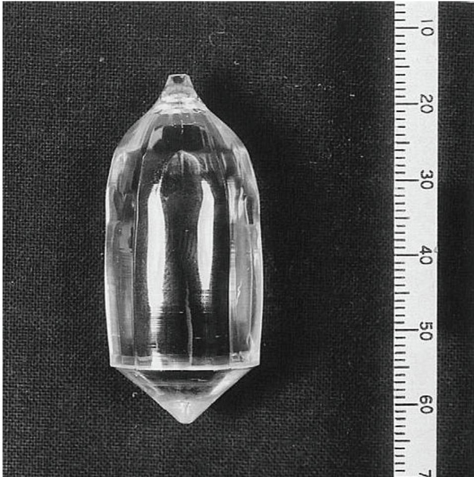
Figure I.2. Photograph of the as-grown  $\text{Lu}_{1.5}\text{Y}_{1.5}\text{Al}_5\text{O}_{12}$  single crystal [42]
