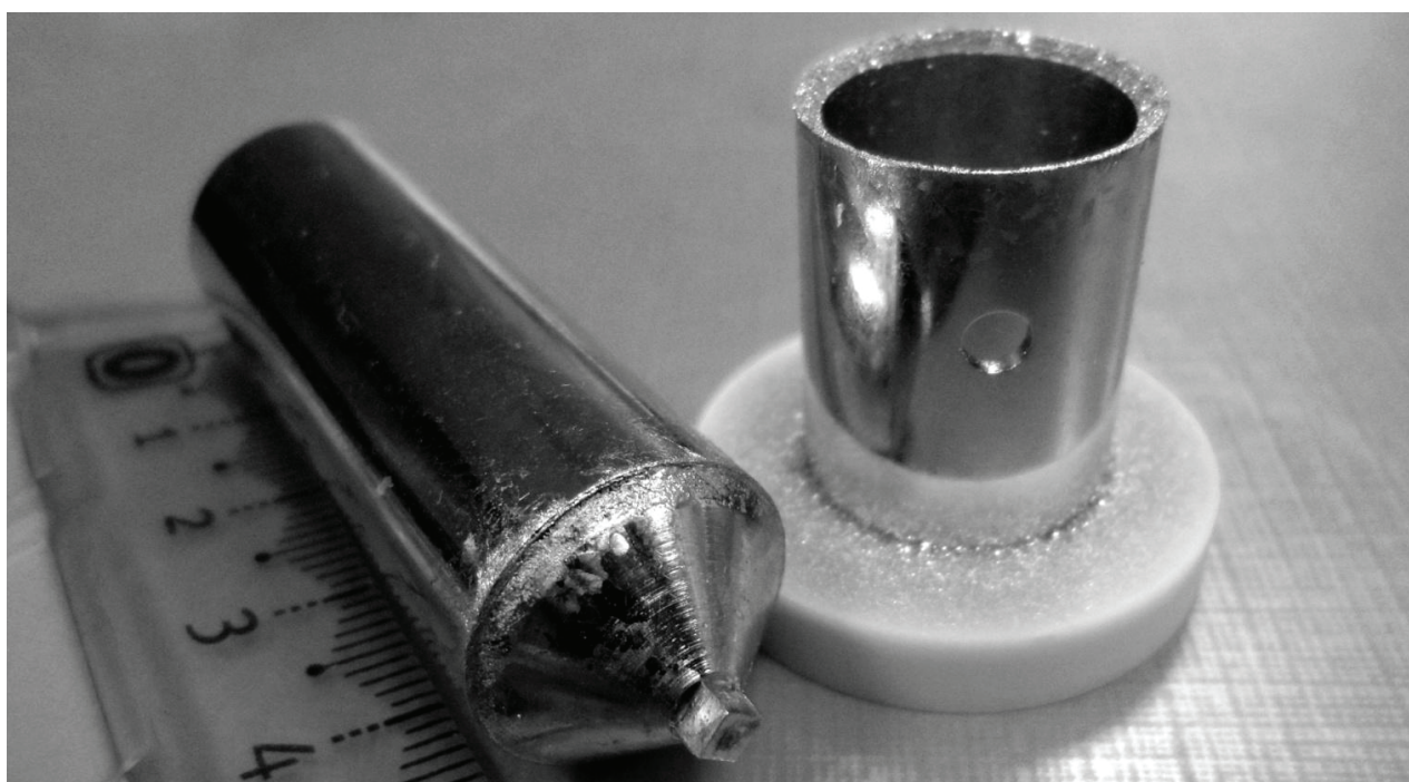
Figure II.1. Ir crucible and afterheater
