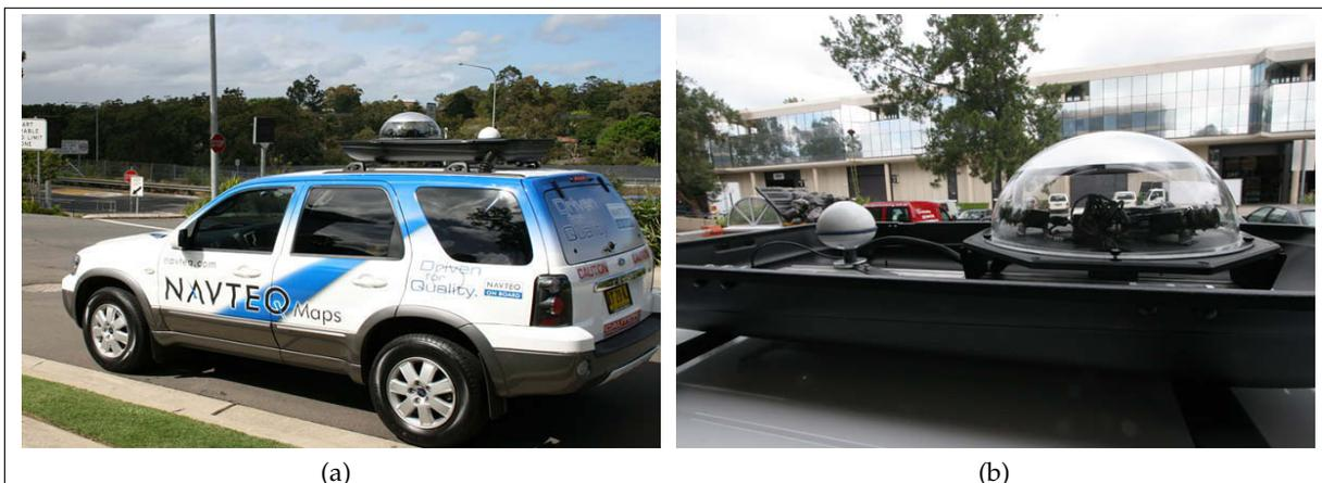
Figure 2.23: (a) NAVTEQ mobile mapping vehicle is equipped with roof-mounted cameras and a GPS antenna. (b) A close-up picture of the array of multiple cameras housed in a transparent perspex cover on the roof of a NAVTEQ mobile mapping vehicle (source [Nav14]).
