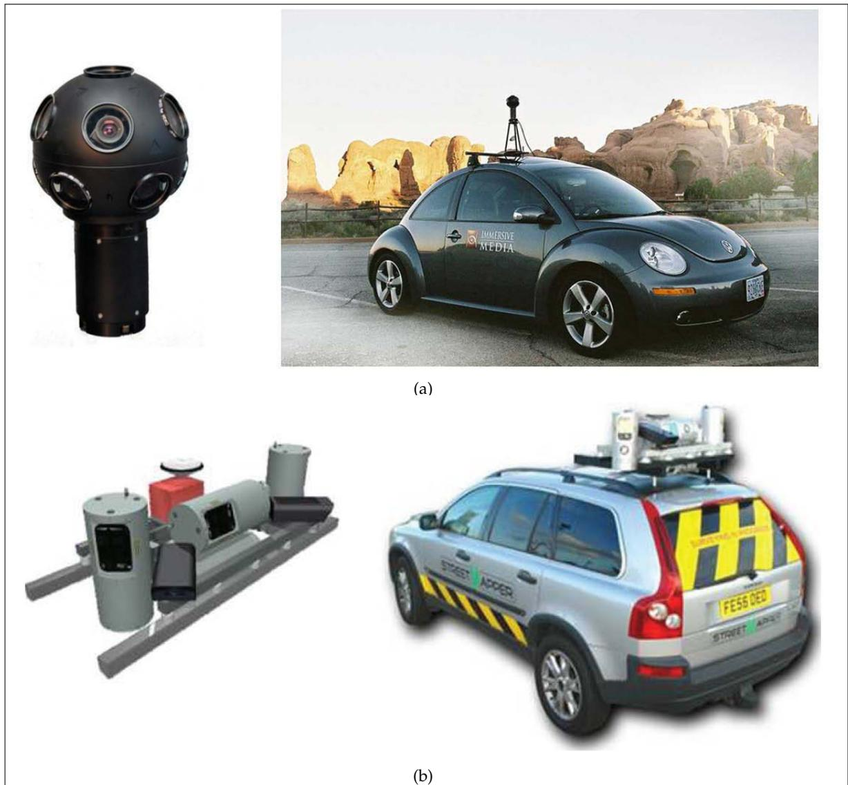
Figure 2.16: (a) Google car with panoramic camera. (b) StreetMapper system of 3DLM with 4 LiDARs (source [3DI14]).
