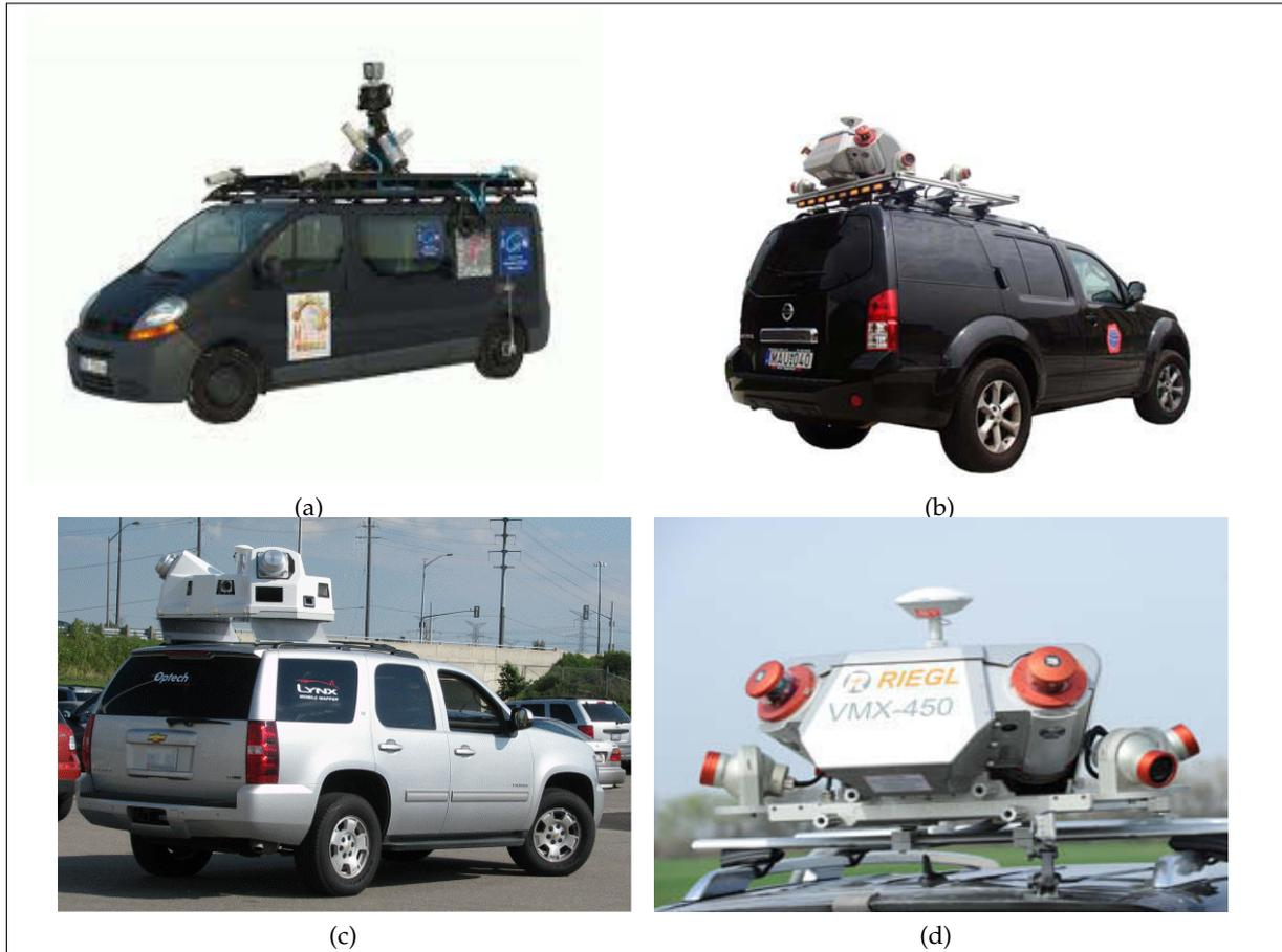
Figure 2.17: (a) STÉRÉOPOLIS II system of (source [Ste14]). (b) Vis center's VizTruck. (c) Lynx SG1 mapping system (source [Opt14]). (d) Riegl VMX-450 mapping system (source [Rie14]).
