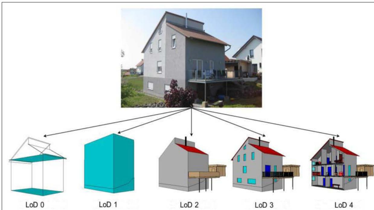
Figure 5.1: Representation of a building using LoD0 - LoD4 [LBG+13].
