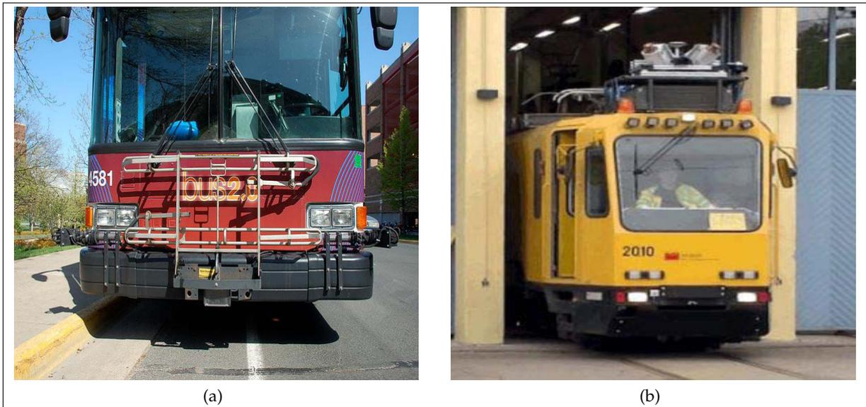
Figure 6.3: (a) & (b) show different sensors mounted on a bus and tramway respectively. These sensors usually include GPS, IMU, cameras and LiDAR sensors.
