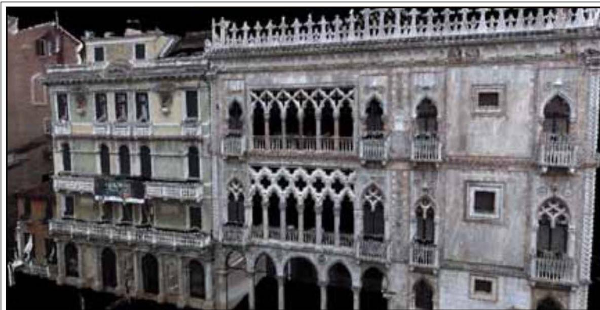
Figure 2.18: True color coded point cloud acquired by Riegl VMX-450 mapping system (source [Rie14]).
