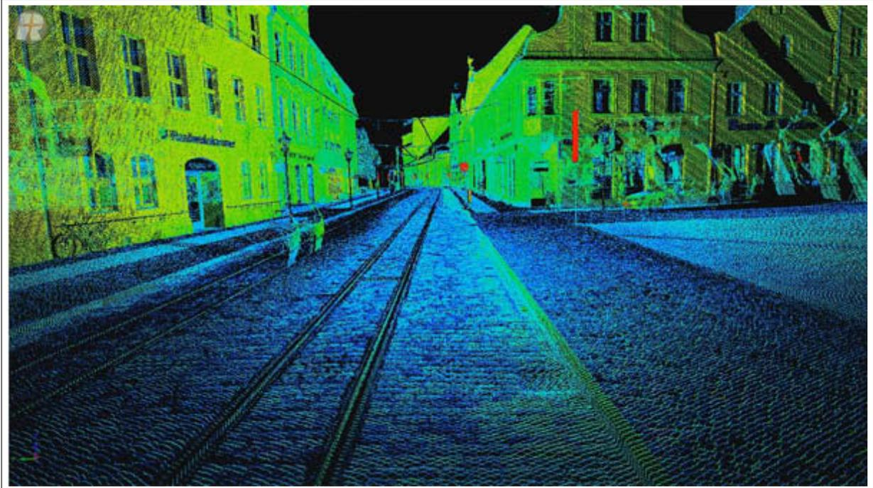
Figure 2.13: 3D data acquired by Riegl MMS VMX-450 using On-the-Fly mode (source [Rie14]).
