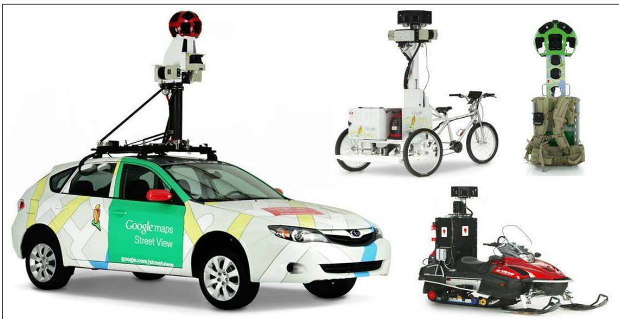
Figure 2.24: Google mobile mapping fleet consisting of mapping vehicles, trikes, snow mobiles and portable backpacks vehicle (source [Goo14]).
