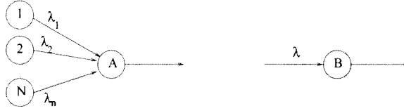
Figure 4.5: Two Models of Input Ports in an OBS Core Node
