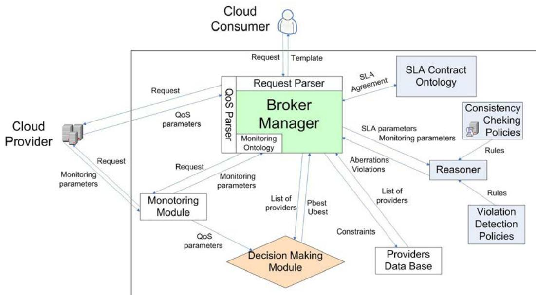
Figure 3.4: Cloud Broker Architecture -
