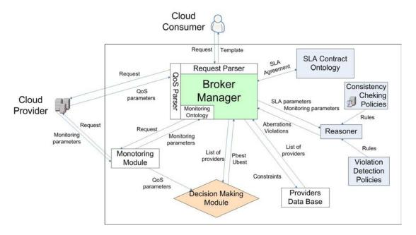
Figure 3.4: Cloud Broker Architecture -
