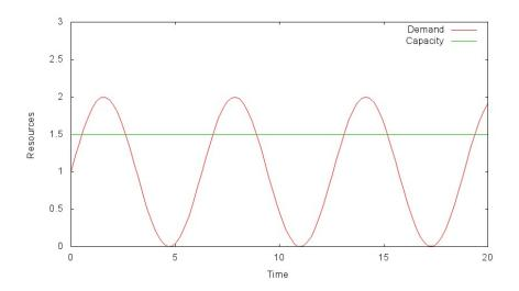
Figure 4.6: Under-provisioning scenario -
