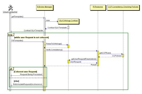
Figure 3.5: Coherent SLA Establishment -
