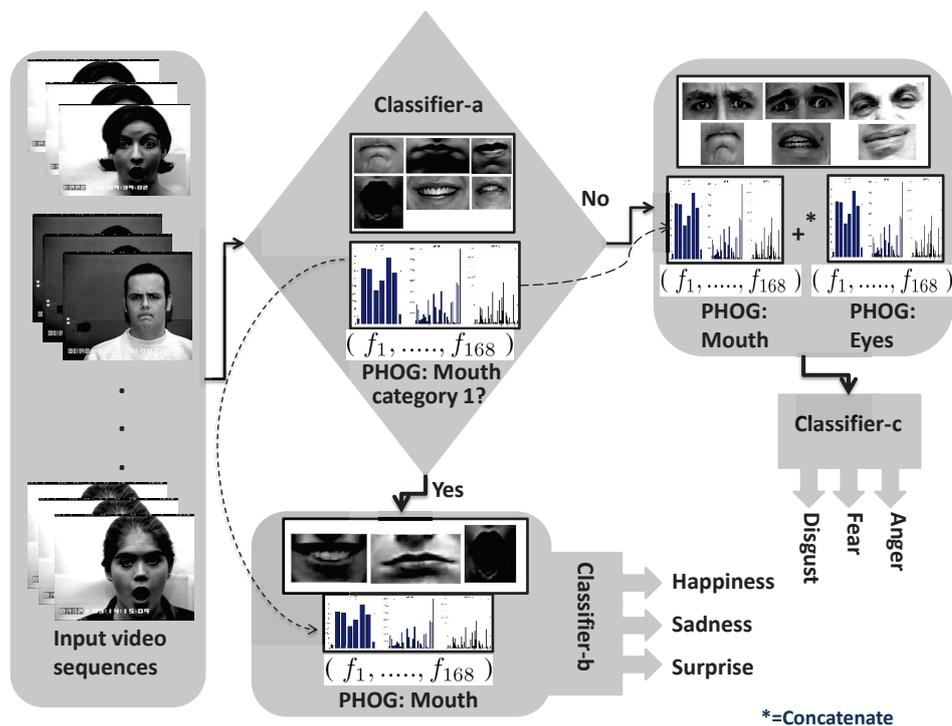
Figure 5.1: Schematic overview of the proposed framework
