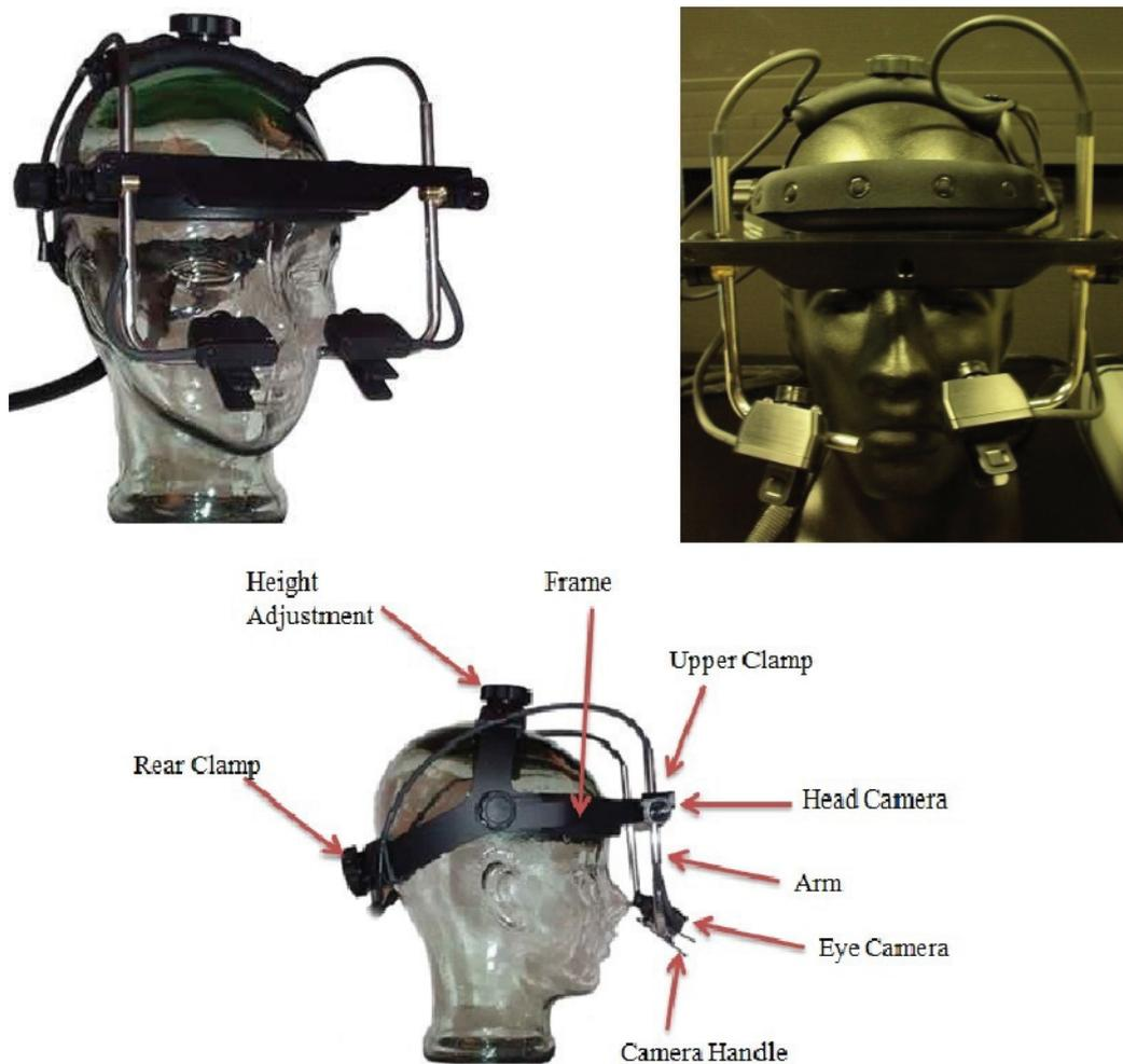
Figure 3.4: Eyelink II, Eye-tracker used in our experiment.
