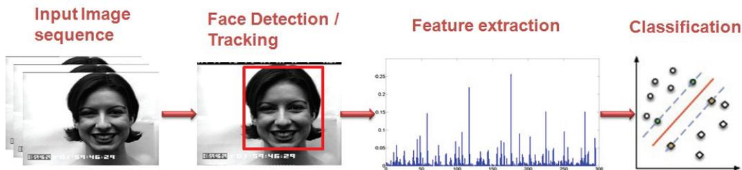
Figure 2.8: Automatic facial expression recognition system pipeline.
