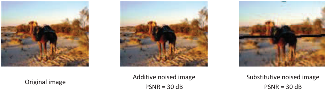
Figure I-11: The same PSNR value (30 dB) may correspond to completely different visual qualities.
