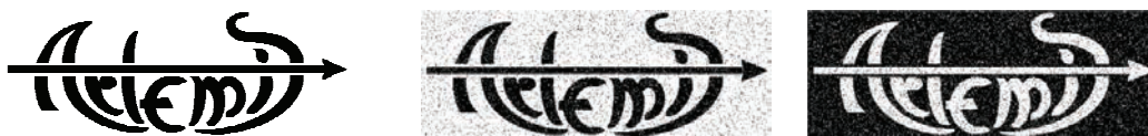
Figure III-8: The ARTEMIS binary logo: original (left), recovered after transcoding (middle) and geometric attacks (right). The original video sequence was encoded at 10 Mbps.
