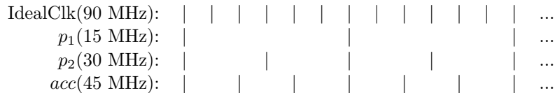
Figure 6.8: Clock modeling of a hardware platform configuration w.r.t an ideal clock. The values in the brackets denote the frequency of the resources.
