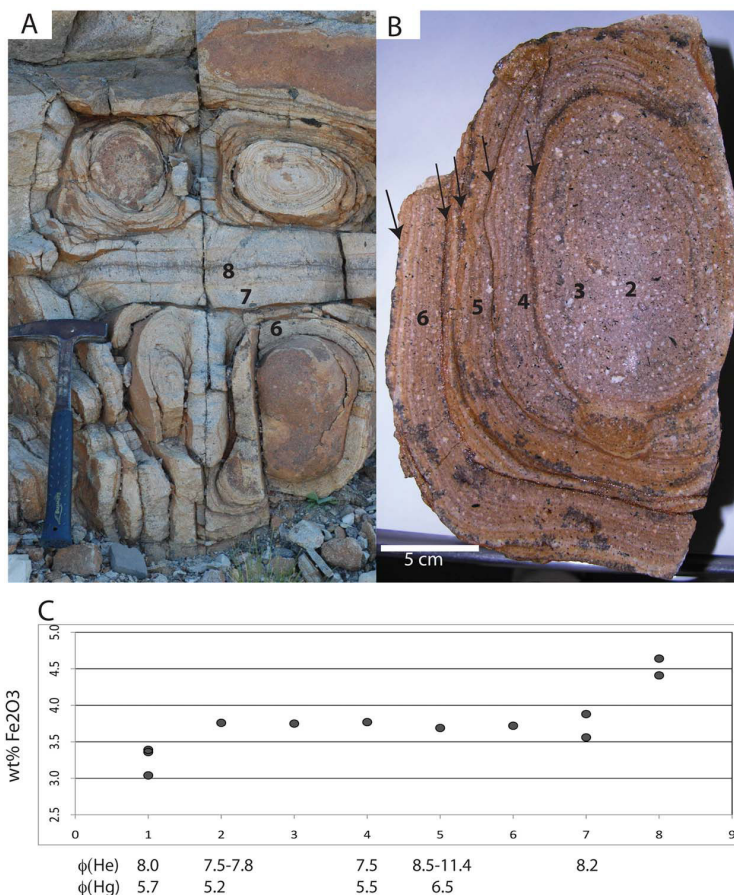
Figure 3. (a) Four corestones rounded by spheroidal weathering. (b) A polished cross section of the stone in the lower-right corner of Figure 3a. This corestone contains numerous Liesegang bands and five “onion-skin” fractures (arrows). Characteristic spacing between rings: Liesegang bands, 2–5 mm; onion-skin fractures, 0.5–3 cm. (c) Bulk rock Fe 2 O 3 contents for the fresh (area 1) and weathered andesites from the corestone shown in Figure 3b. Numbers correspond to locations on the corestone. The fresh andesites (area 1) are from the same outcrop a few meters away from these corestones. He- and Hg-porosimetry performed for approximately 2 cm 3 samples from the unfractured core (areas 2 and 3) and for Liesegang banded (but macroscopically unfractured) areas 5 and 6. CT scans were carried out on somewhat smaller (0.1–0.2 cm 3 ) samples collected between layers 3 and 4 (innermost “onion-skin” fracture) and between layers 4 and 5 (second innermost fracture). He- and Hg-porosity values are given for samples cut out from the various locations indicated by numbers in Figures 3a and 3b.
