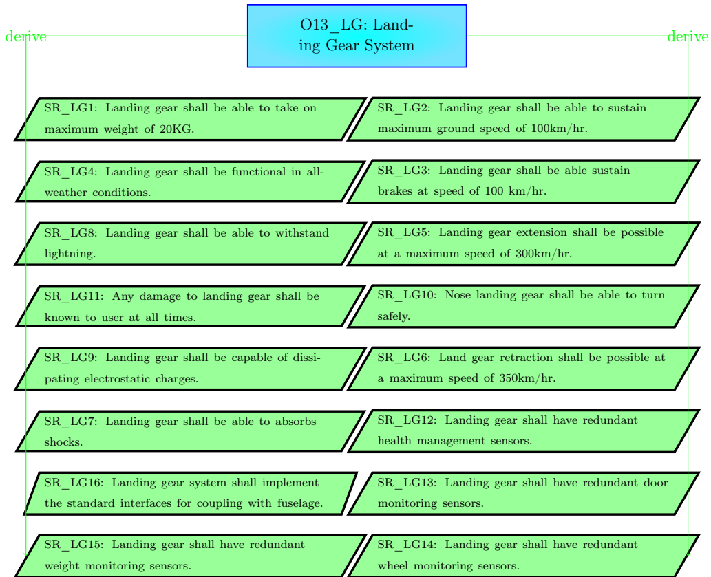
Figure 5.19: IBIS Landing Gear System Requirements
