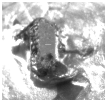
Figure 5.1.2 Camera view of Cd_6Yb single crystal glued on the sample holder.
