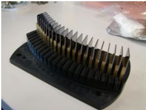
Figure 2.3.3 A view of the multi-analyzer detector used at Crystal beamline, Soleil, France.
