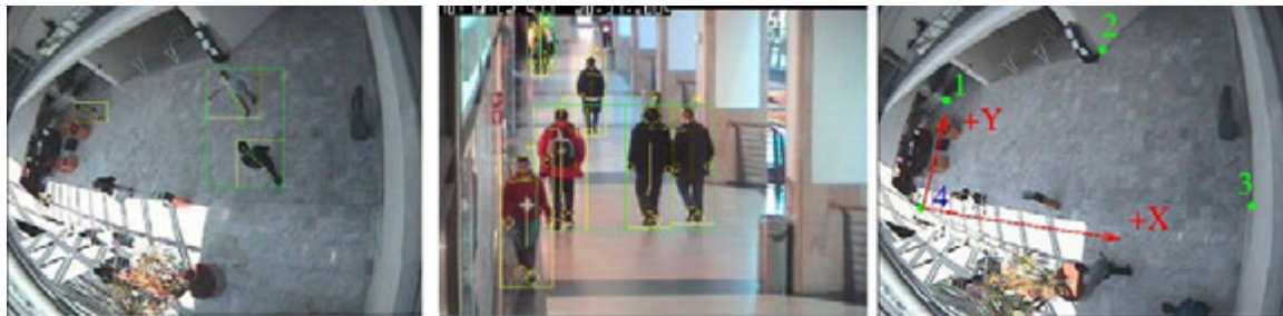
FIGURE 2.13: Sample frames from the CAVIAR dataset ( Caviar (2004) ) with ground truth for pedestrians with body parts (in yellow), groups of people (green boxes), and ground plane detection in the last image on the right.
