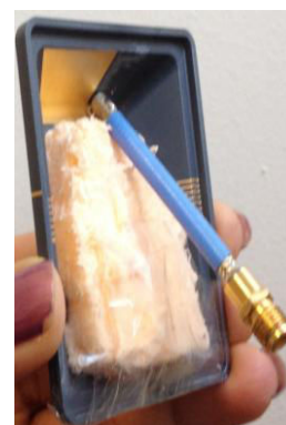
Fig. 4.63 : Three dimensional PIFA antenna on LCP Vectra E820i, (a) simulated structure and (b) fabricated photo.
