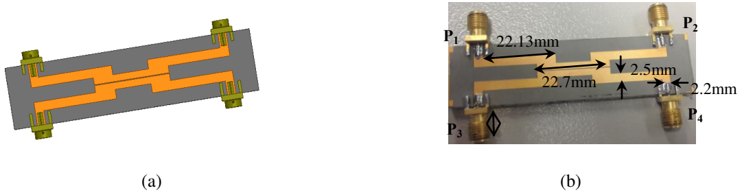
Fig. 6.21 : Three sections directional coupler realized on High K material, (a) its simulated structure and (b) the fabricated device.
