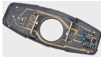
Fig. 2.16 : MID lighting module for vehicles.
