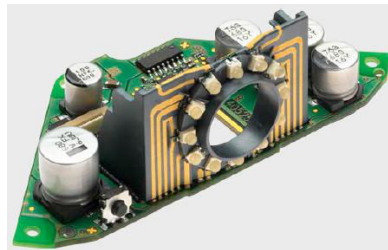
Fig. 2.23 : MID safety camera system from SICK AG.
