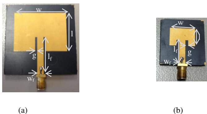
Fig. 4.58 : LDS MID antenna structures on LCP Vectra E820i: (a) at 2.63 GHz and (b) at 5.8 GHz.
