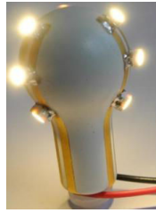
Fig. 2.20 : LED lamp integrated with LDS technology.
