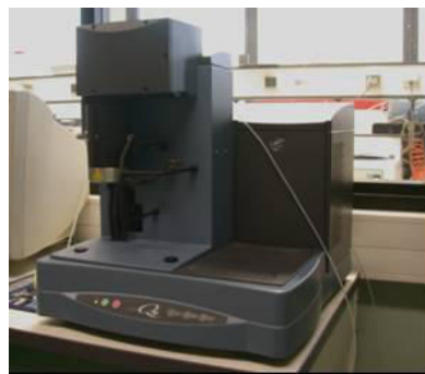
Fig. 3.2 : Photograph of the equipment of TGA.
