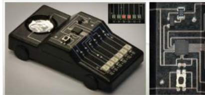
Fig. 2.18 : 3D MID with integrated sensor-Automotive tank level filling sensor.
