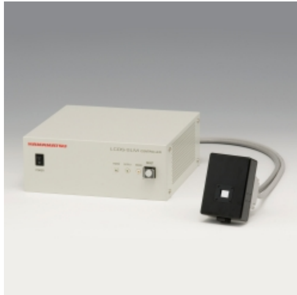
Figure 7.5: Liquid-Crystal-on-Silicon Spatial Light Modulator (LCOS-SLM) device used. It is a Hamamatsu® LCOS-SLM X10468 series, for 1064nm light, whose active area consists of 792 \times 600 pixels, with pixel size 20\mu m \times 20\mu m .
