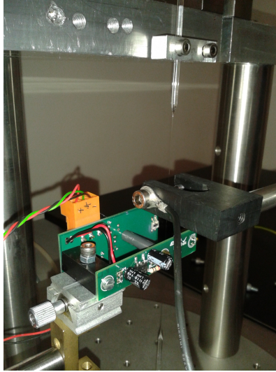
Figure 5.14: The picture shows the system for the loss angle measurements. The exciter (in black), the fiber held by its clamping system (see fig. 5.12) and the shadowmeter with the alimeted led and photodiode.
