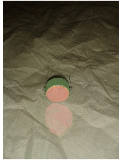
(b) The mirror suspends by one Niobium wire.
