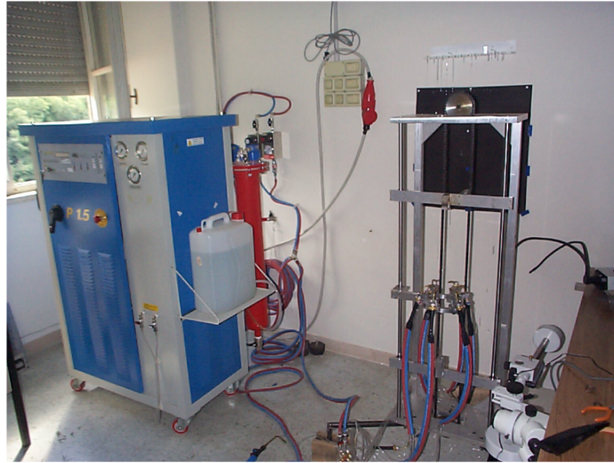
Figure 5.7: Machine for the production of the oxyhydrogen flames by electrolysis of distilled water, on the left. On the right the machine for the production of the silica fibers.
