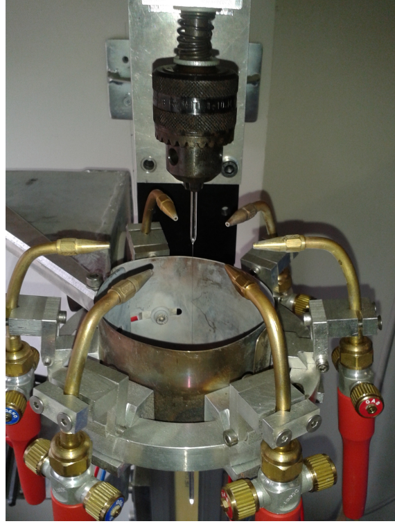
Figure 5.9: The system with the crown of 6 hooks with nozzle for flame. The pulled fiber is held in the middle of the crown. It is visible the thicker part of the original silica seed.
