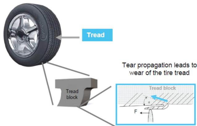
**Figure 6: Relationship between resistance to tear propagation and tire tread wear.**
