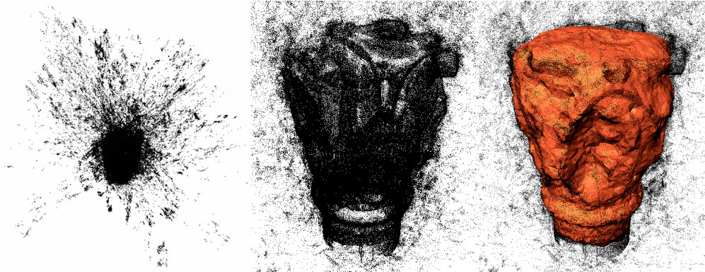
Figure 5.25: Noise and structured outliers. Left: raw point cloud. Middle: closeup on point cloud. Right: closeup on point cloud & reconstruction.
