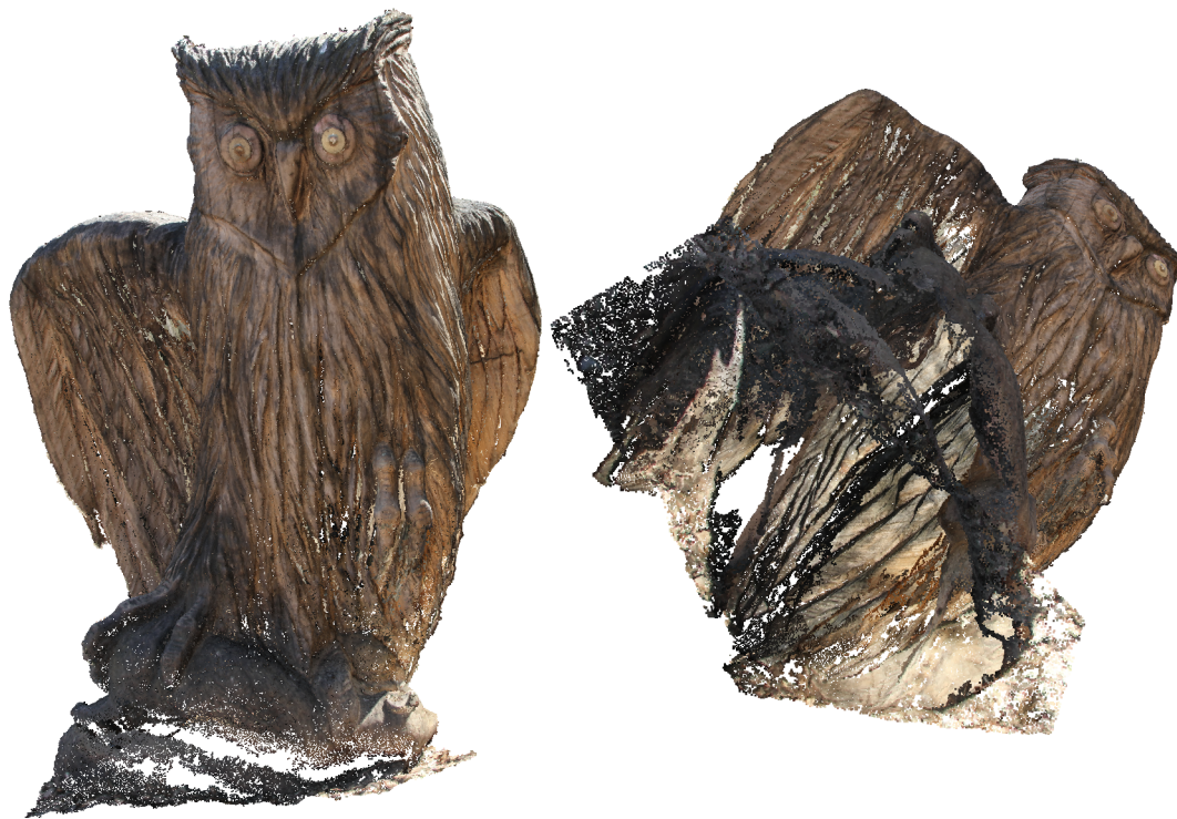
Figure 1.8: Owl point cloud with missing data on the bottom (courtesy EPFL Computer Graphics and Geometry Laboratory [2])
