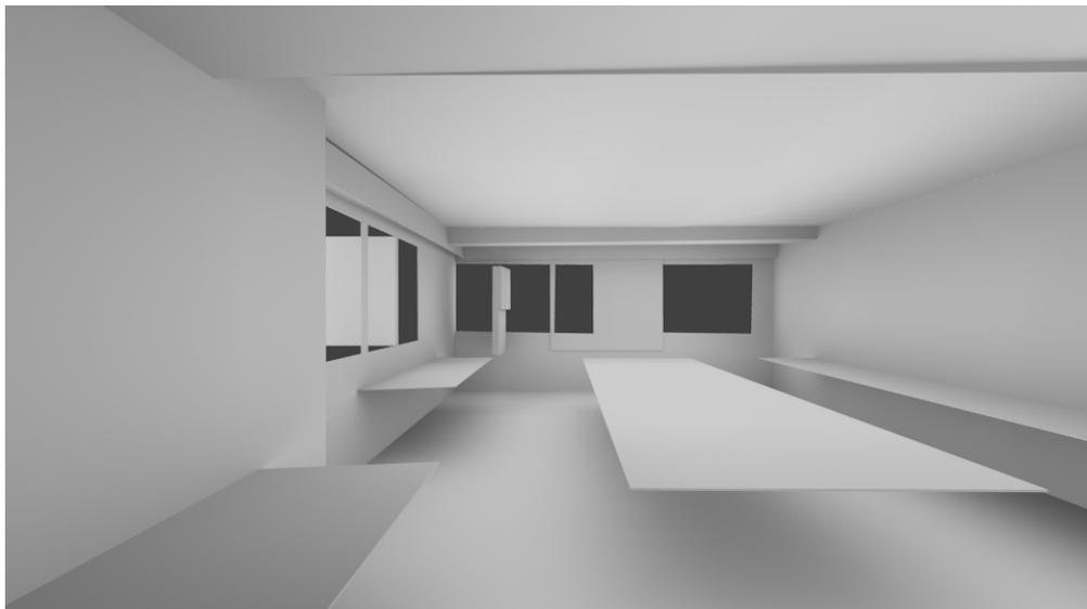
Figure 6.3: **Regularized algorithm** [16]. The output of this algorithm is a coarse piecewise-planar mesh thanks to the regularization energy penalizing overly complex shapes.
