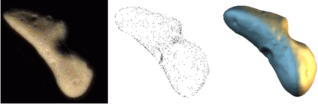
Figure 2.10: Radial basis functions [21]. Left: photo of asteroid Eros. Middle: input point cloud with variable sampling density. Right: reconstruction using RBF.
