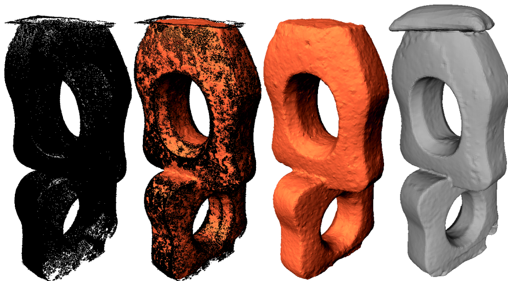
Figure 5.18: Low noise. From left to right: raw point cloud; point cloud & reconstruction; reconstruction only; Poisson reconstruction.
