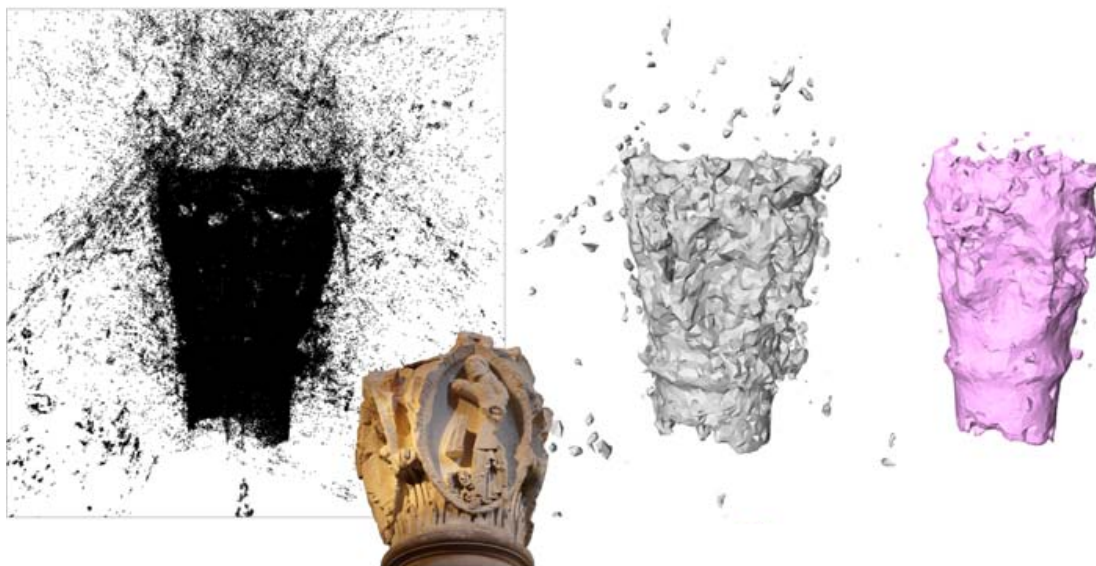
Figure 2.9: “ Signing the unsigned ” algorithm [64]. Left: input point cloud and photo. Middle: estimation of the inferred surface. Right: reconstructed surface.
