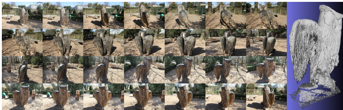
Figure 1.3: Point cloud acquired by photogrammetry. About 30 photos of the owl statue from the EPFL Repository [2] have been taken to produce the point cloud shown on the right (displayed in MeshLab ).
