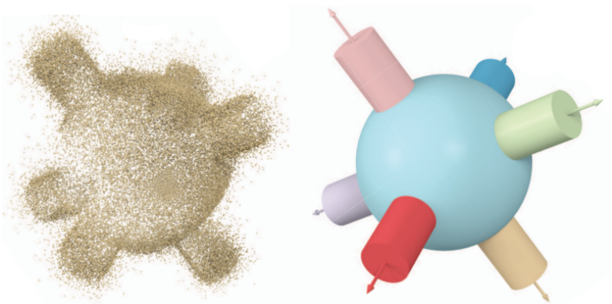
Figure 2.12: GlobFit algorithm [57]. Primitives are fit to a point cloud with non-uniform sampling density.
