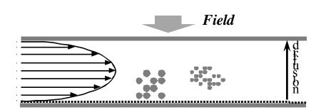
Figure 1.4 Basic separation principle of flow field flow fractionation
