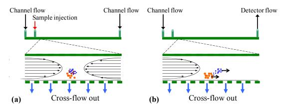
Figure 2.10 Principle of the separation of macromolecules by FIFFF. (A) Injection and focusing/relaxation step; (B) Elution step
