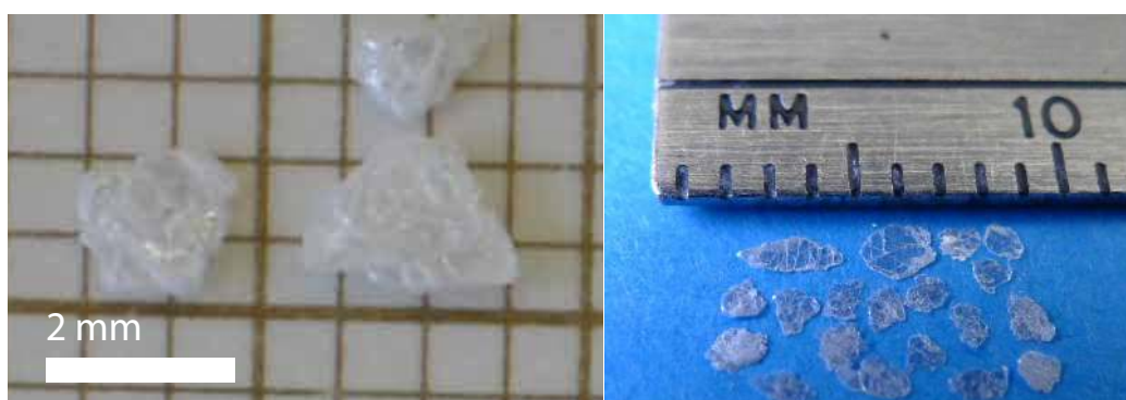
Figure 2.2: Left: picture of h-BN crystals synthesized by high pressure and high temperature process at NIMS, Tsukuba, Japan [34]. Right: crystal synthesized by a new commercial provider (HQ-graphene http://www.hqgraphene.com/ ). Both crystals are few millimeter sized and display a very high crystallinity level.
