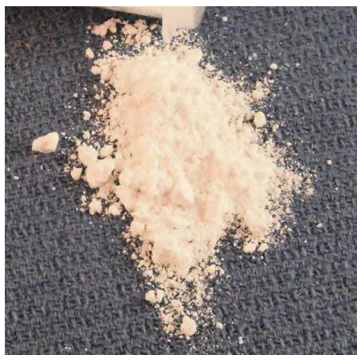
Figure 2.3: white micrometer sized powder of h -BN sold by a chemical provider
