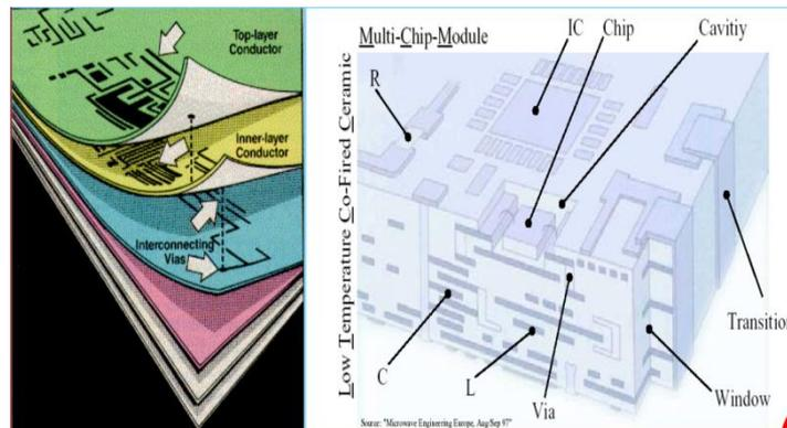
Fig.48 : Technologie LTCC '' source : Microwave engineering Europe, Aug/Sep 97''
